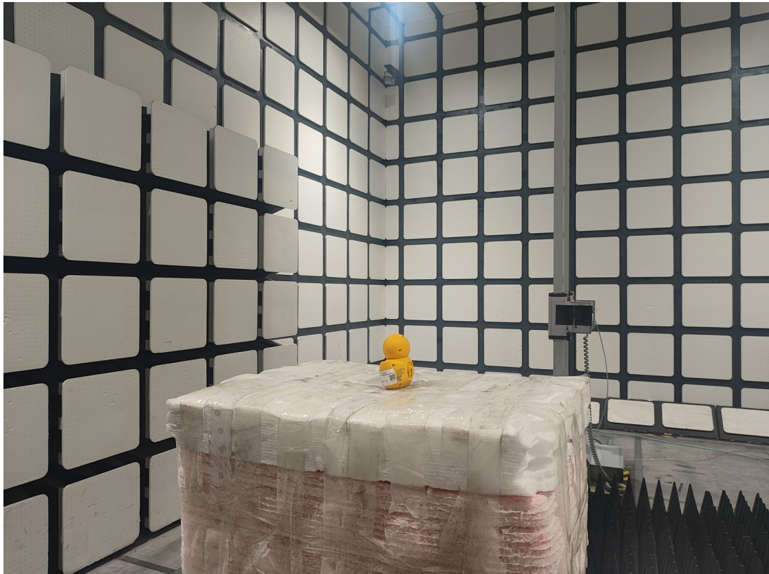
Radiated Emissions View (18-25 GHz)
