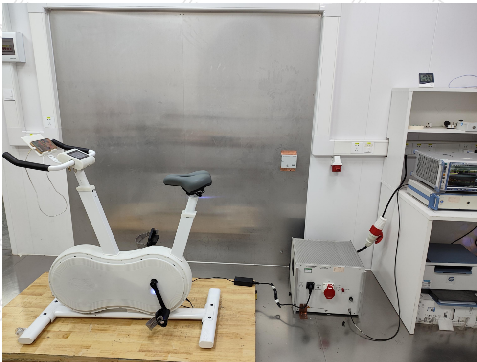
Photo of Conducted Emission Measurement
