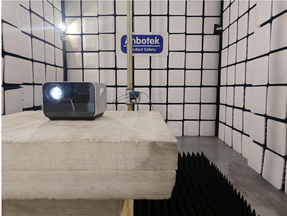
Photo of Radiation Emission Test (above 1GHz)
