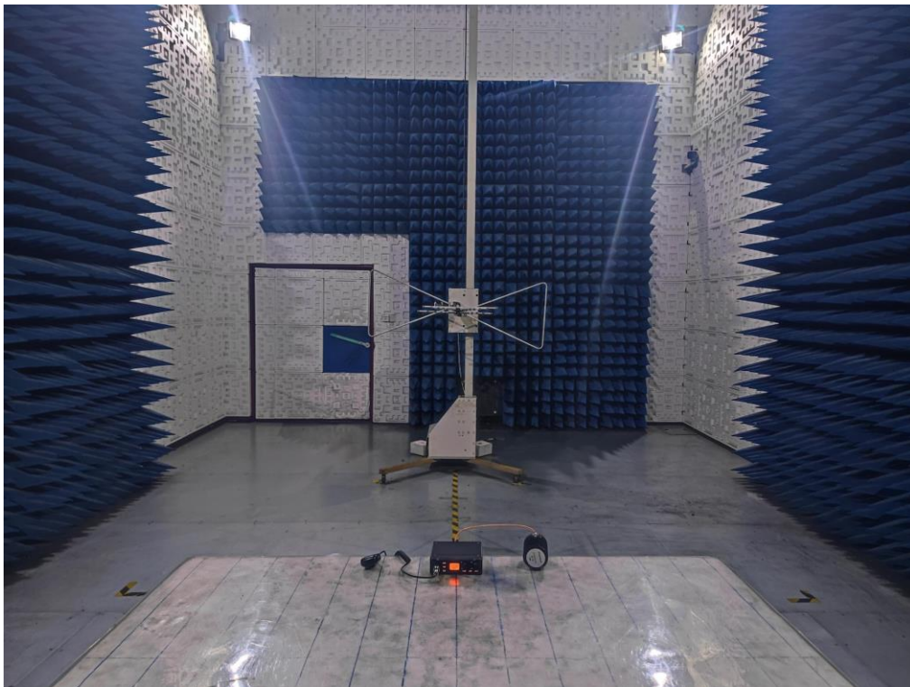
RADIATED EMISSION TEST SETUP BELOW 1GHz
