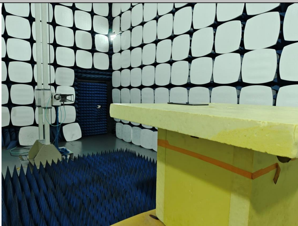
Radiated Emission, Above 1GHz
