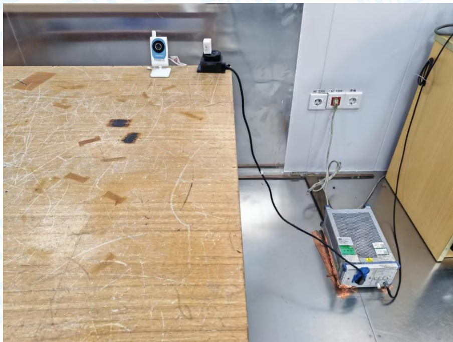
Photo of Setup for Radiated Emission (30MHz~1GHz)
