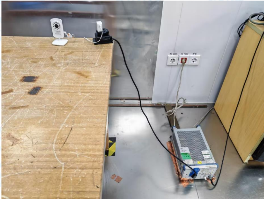
Photo of Setup for Radiated Emission (30MHz~1GHz)
