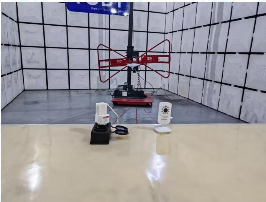
Photo of Setup for Radiated Emission (30MHz~1GHz)
