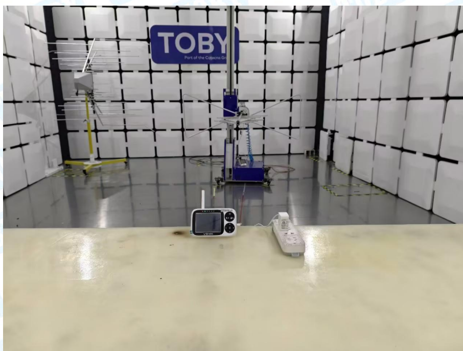
Photo of Setup for Radiated Emission (30MHz~1GHz)
