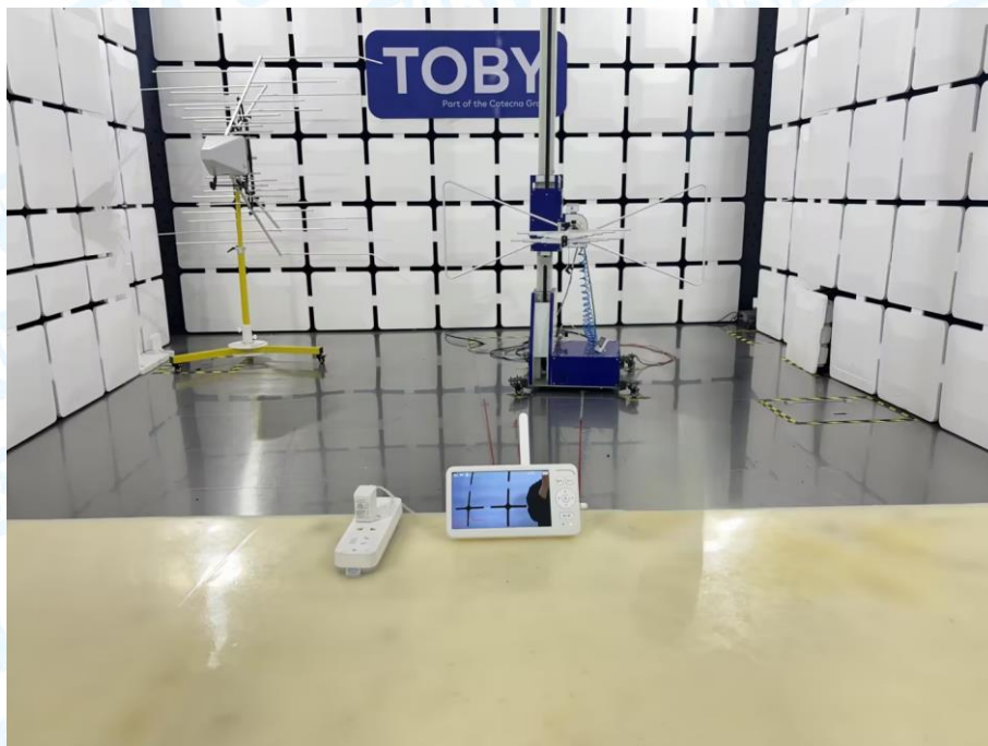
Photo of Setup for Radiated Emission (30MHz~1GHz)
