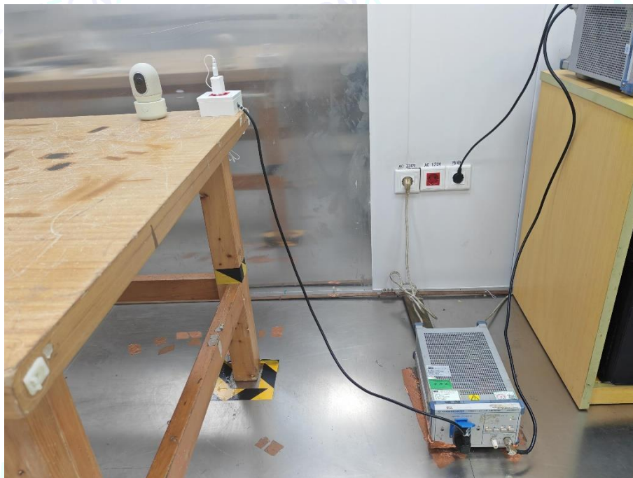
Photo of Setup for Radiated Emission (30MHz~1GHz)
