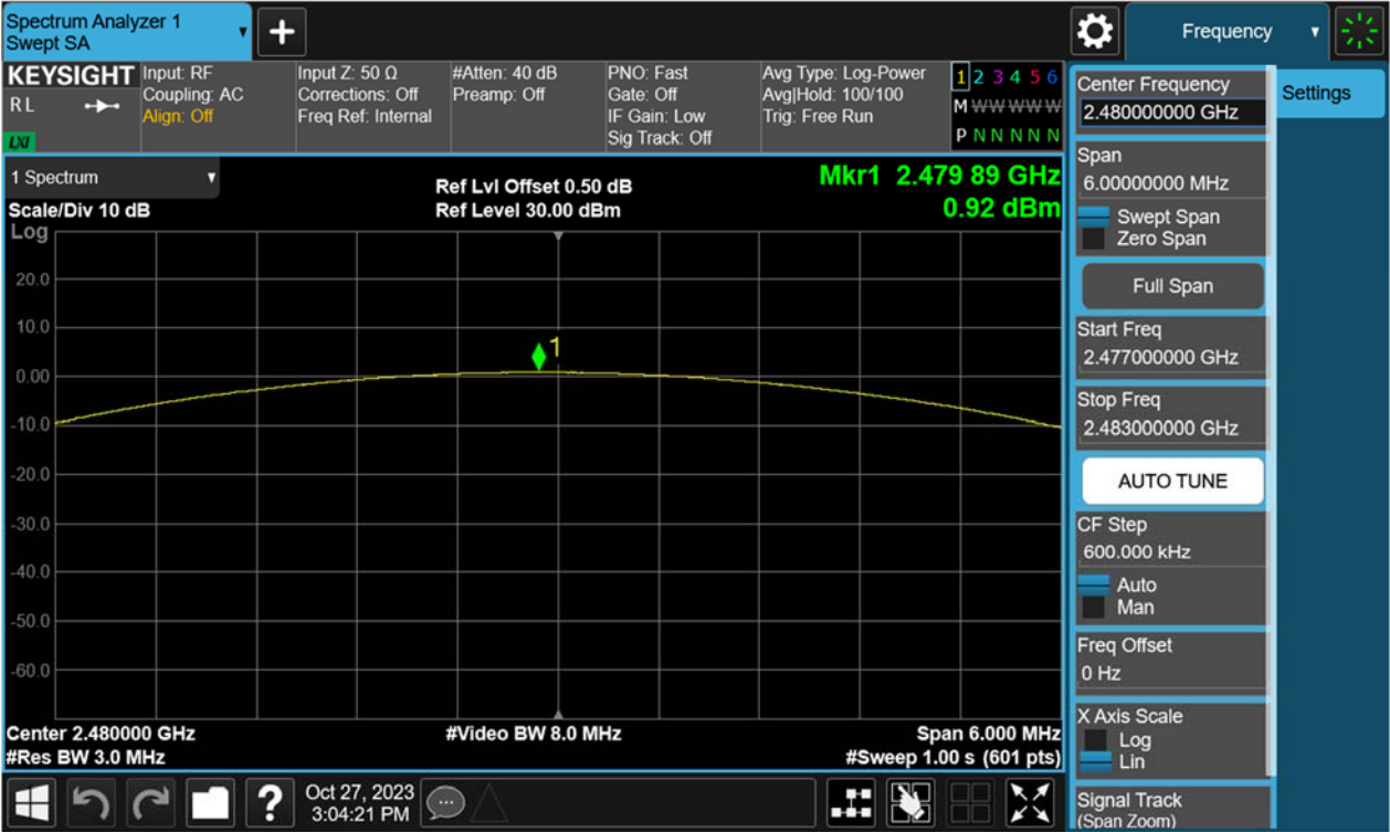
Figure 9: Maximum Peak Output Power, 2480MHz, 8-DPSK
