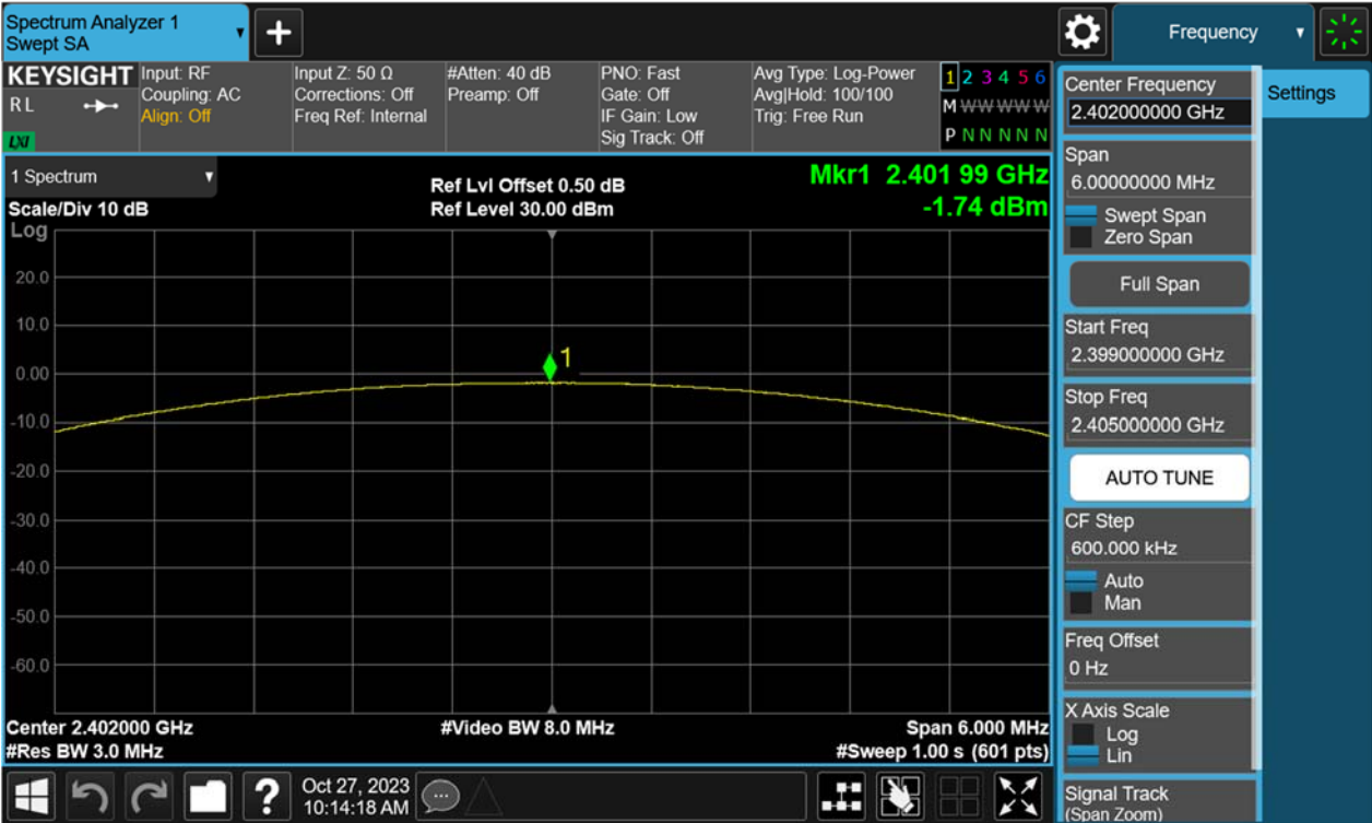
Figure 4: Maximum Peak Output Power, 2402MHz, \pi/4 -DQPSK
