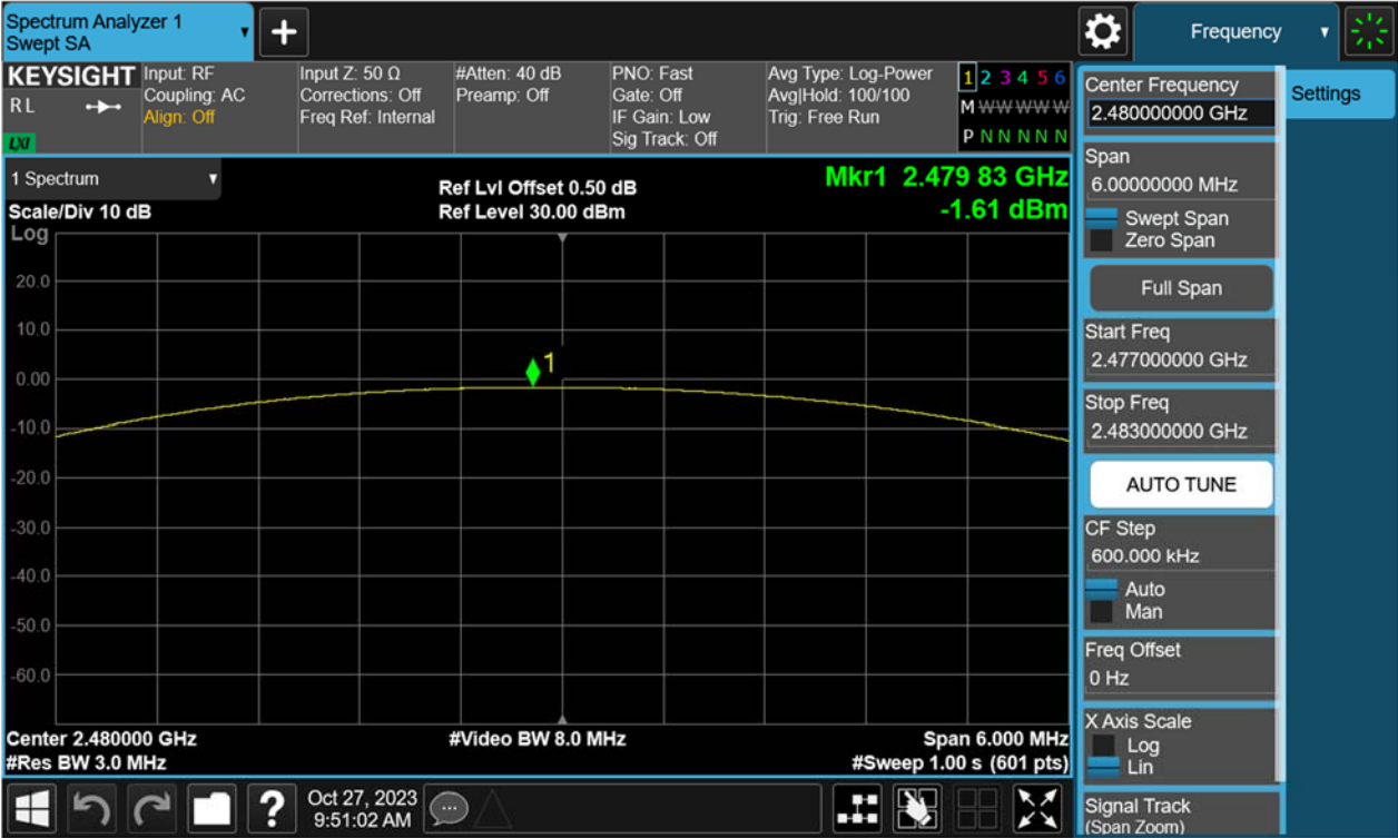
Figure 4: Maximum Peak Output Power, 2402MHz, \pi/4 -DQPSK
