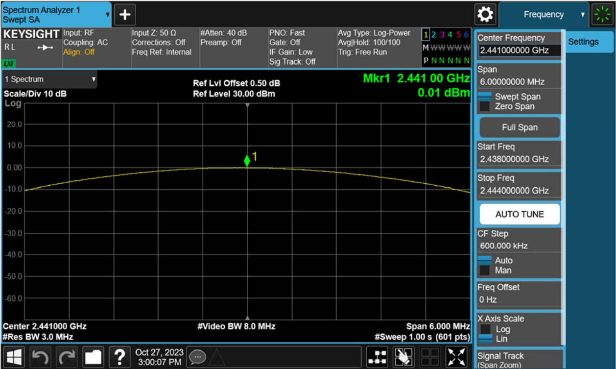
Figure 8: Maximum Peak Output Power, 2441MHz, 8-DPSK
