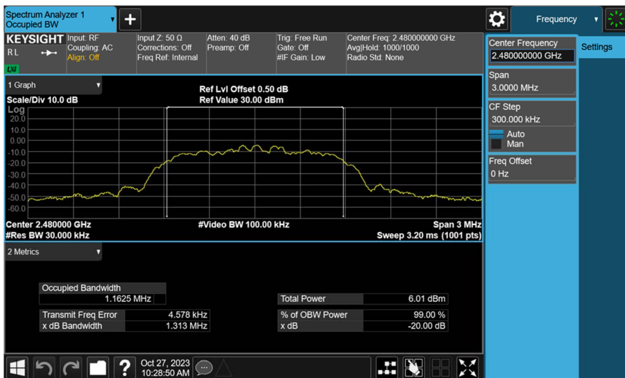
Figure 15: 20dB Bandwidth and 99% Bandwidth, 2480MHz, \pi/4 -DQPSK
