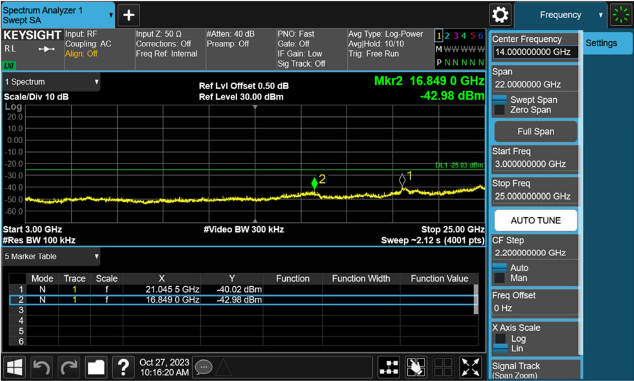
Figure 23: Conducted Spurious Emission & Authorized-band band-edge, 2441MHz, \pi/4 -DQPSK Carrier Level
