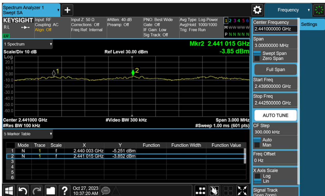
Figure 32: Hopping Frequency Separation, Hopping Mode, \pi/4 -DQPSK
