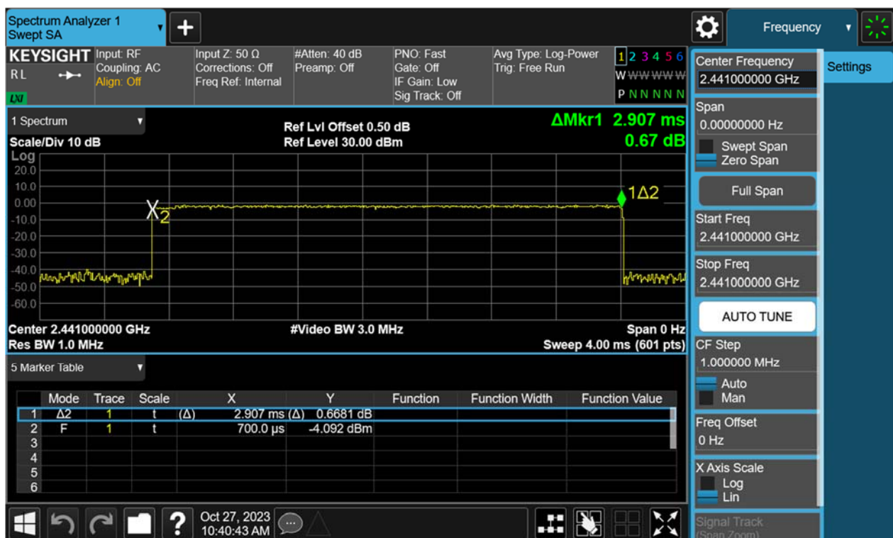
Figure 42: Time of Occupancy, 2441MHz, \pi/4 -DQPSK DH5
