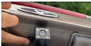
K.Secure the rear camera above the center of the license plate frame.
