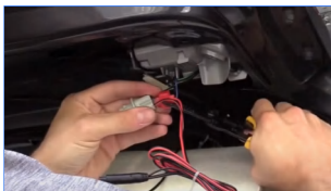
I.Connect the red cable of the rear camera to the positive terminal of the reversing light.
