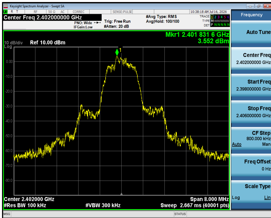
Tx. Spurious NVNT 2-DH1 2402MHz Ant1 Ref
