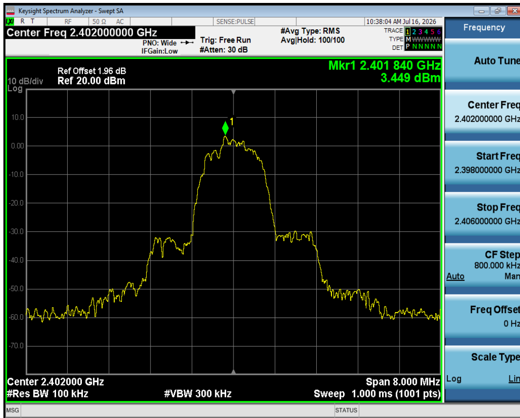
Band Edge NVNT 2-DH1 2402MHz Ant1 No-Hopping Ref
