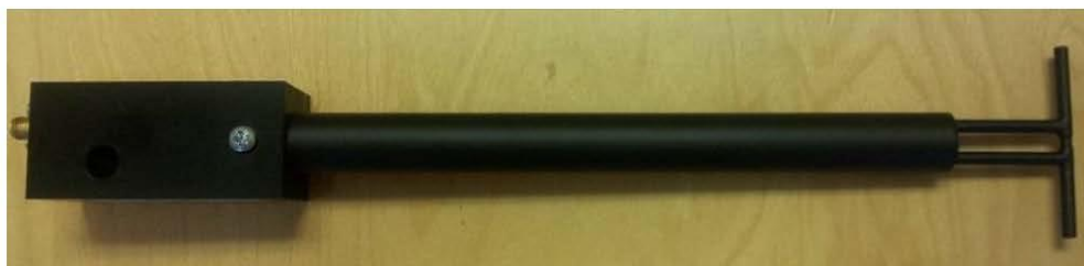
Figure 1 – MVG COMOSAR Validation Dipole
