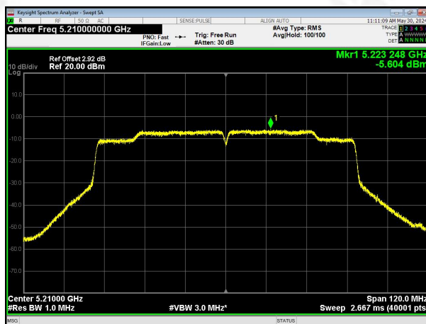
ANT2 (802.11ac80) PSD plot on channel 42
