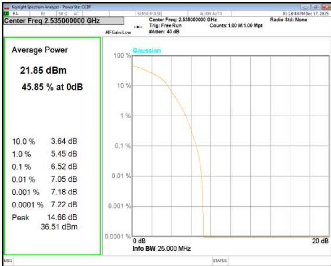
Band7 16QAM BW=15MHz Channel=21375 RB Size=1 Position=#0
