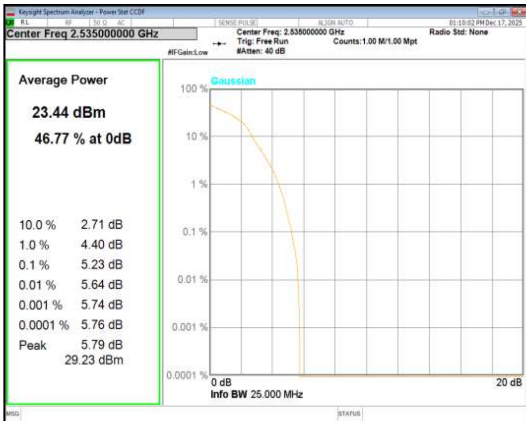
Band7 16QAM BW=10MHz Channel=21400 RB Size=1 Position=#0
