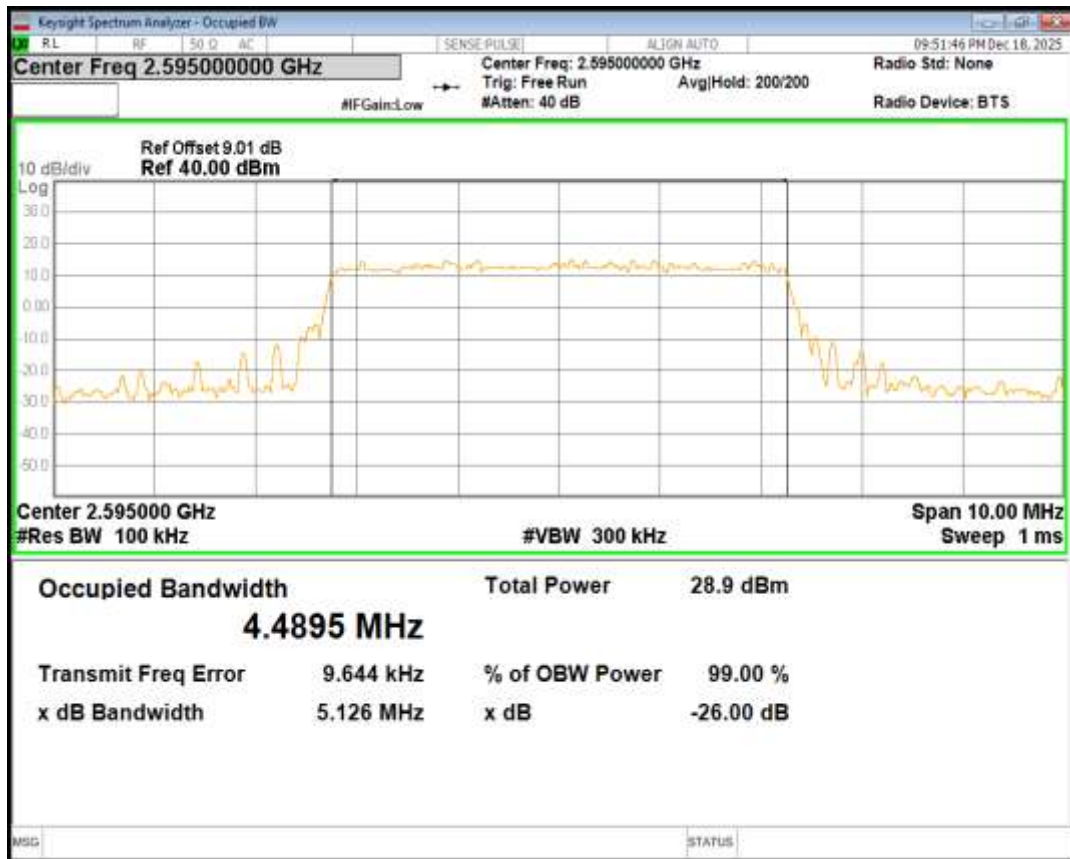
Band38 16QAM BW=5MHz Channel=38225 RB Size=25 Position=#0
