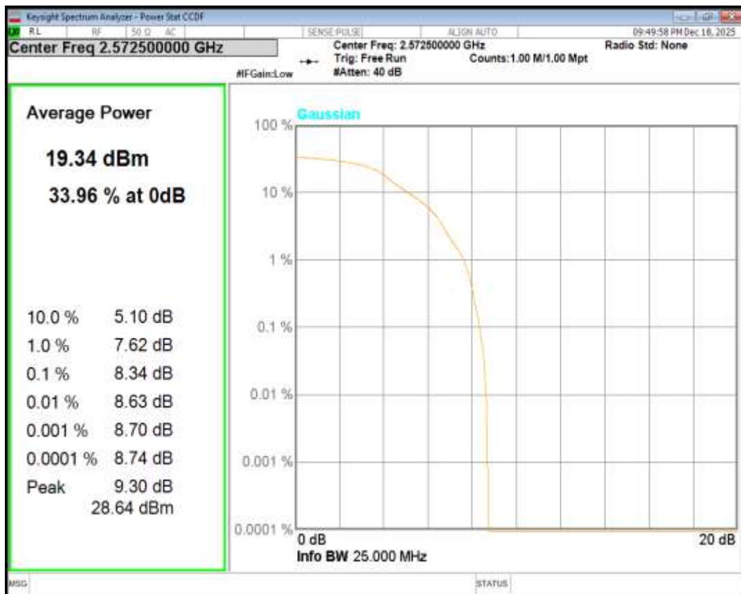
Band38 QPSK BW=5MHz Channel=38000 RB Size=1 Position=#0
