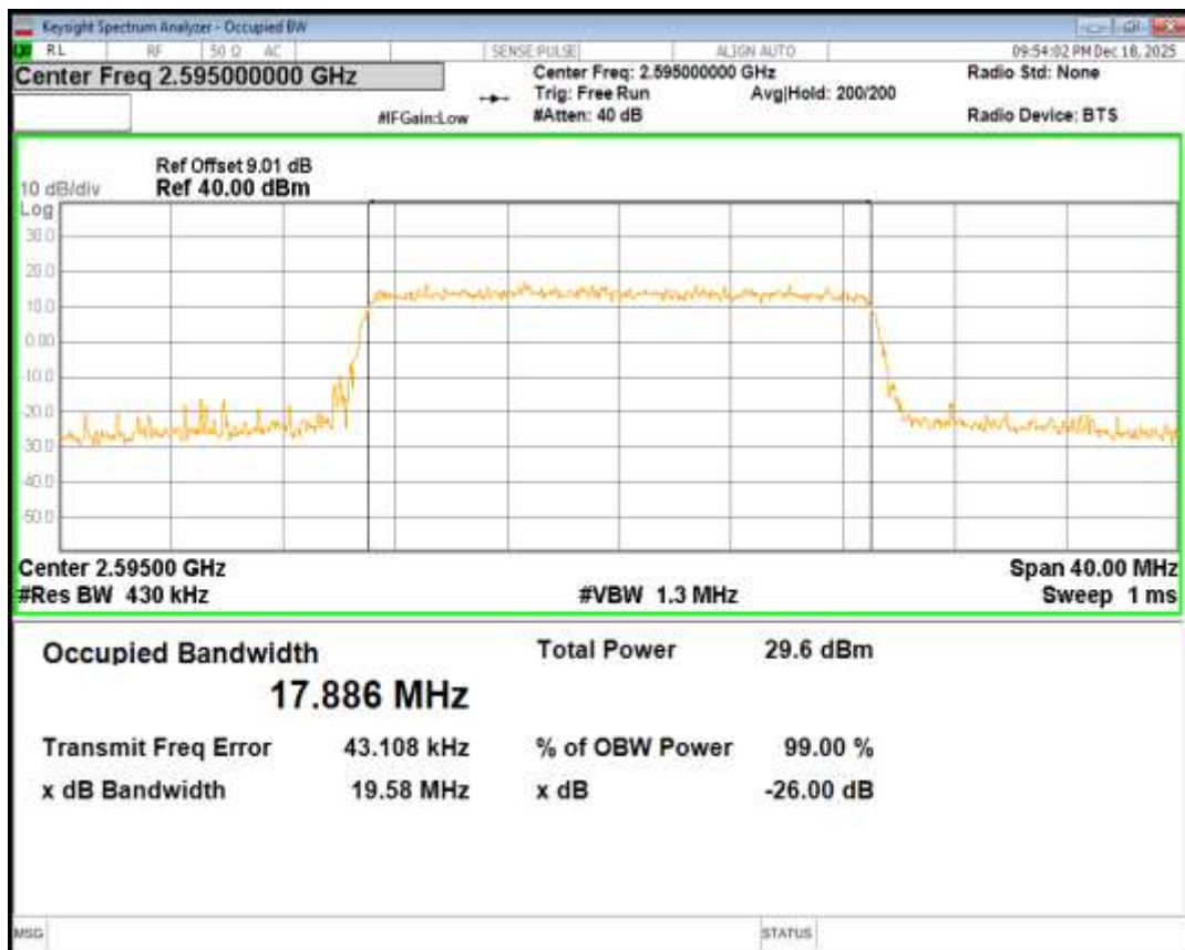
Band38 QPSK BW=20MHz Channel=38150 RB Size=100 Position=#0
