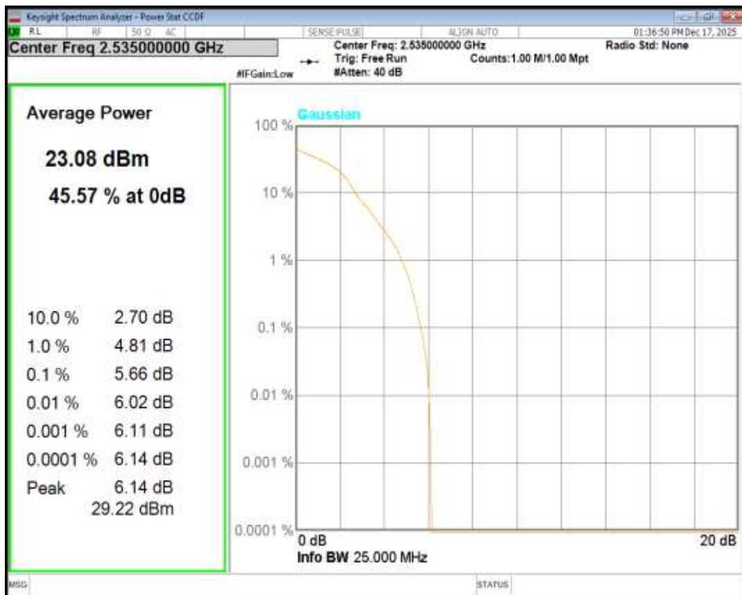
Band7 16QAM BW=20MHz Channel=21350 RB Size=1 Position=#0
