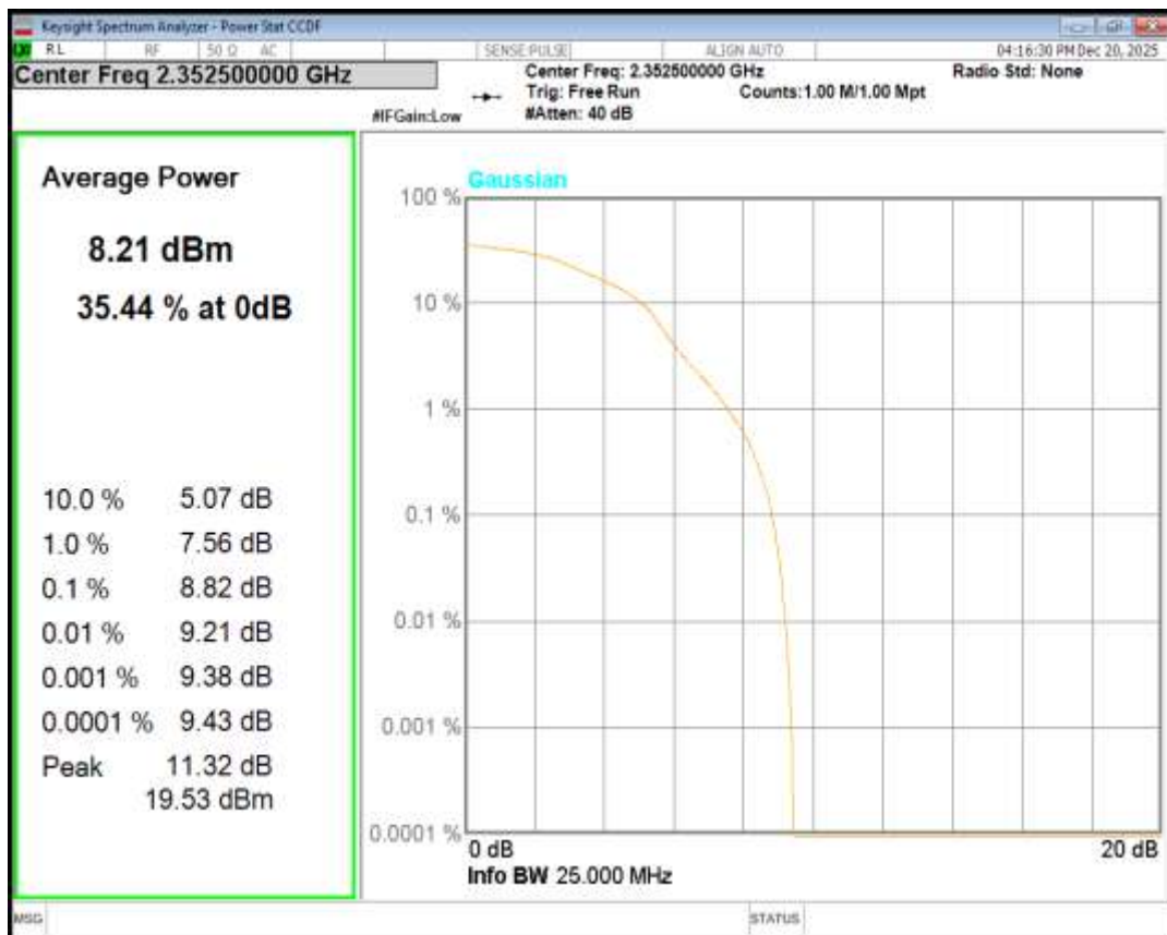
Band40(2350-2360) 16QAM BW=5MHz Channel=39200 RB Size=1 Position=#0
