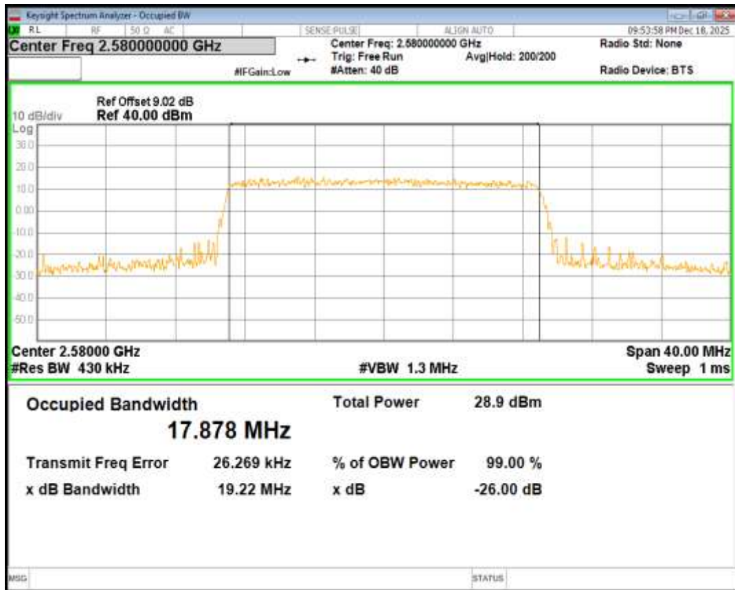
Band38 16QAM BW=20MHz Channel=38000 RB Size=100 Position=#0
