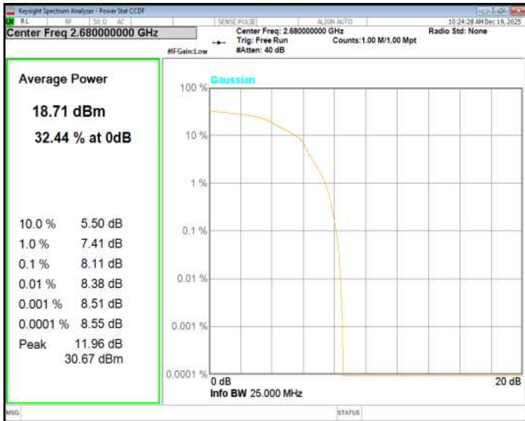
Band41 16QAM BW=5MHz Channel=39675 RB Size=1 Position=#0
