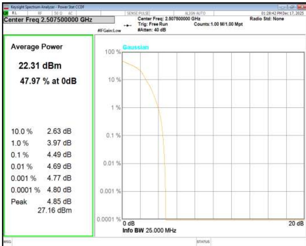
Band7 16QAM BW=15MHz Channel=21100 RB Size=1 Position=#0
