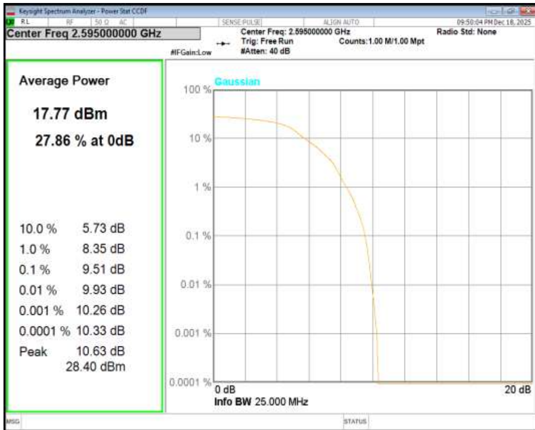
Band38 QPSK BW=5MHz Channel=38225 RB Size=1 Position=#0
