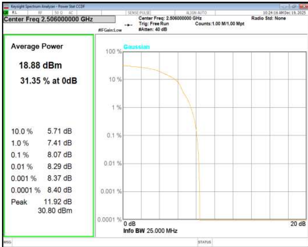
Band41 16QAM BW=20MHz Channel=40620 RB Size=1 Position=#0
