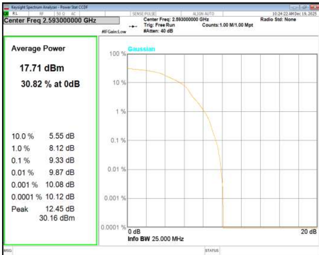
Band41 16QAM BW=20MHz Channel=41490 RB Size=1 Position=#0
