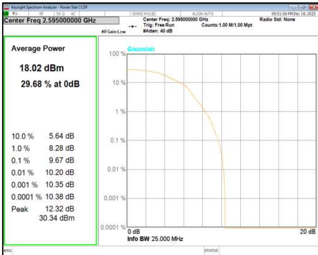
Band38 16QAM BW=20MHz Channel=38150 RB Size=1 Position=#0
