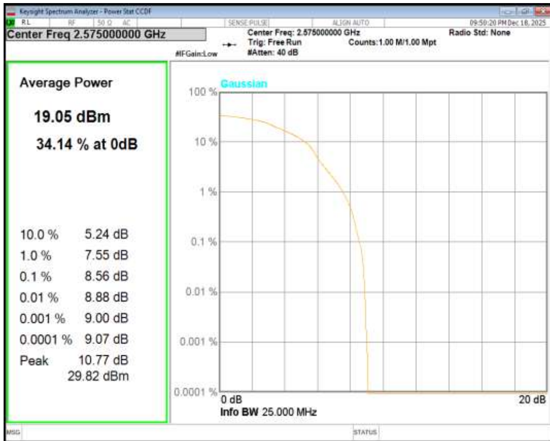
Band38 16QAM BW=10MHz Channel=38000 RB Size=1 Position=#0
