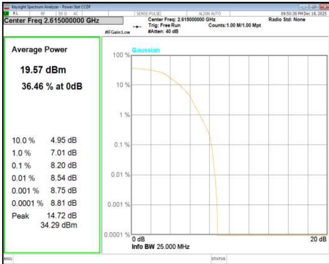
Band38 QPSK BW=15MHz Channel=37825 RB Size=1 Position=#0
