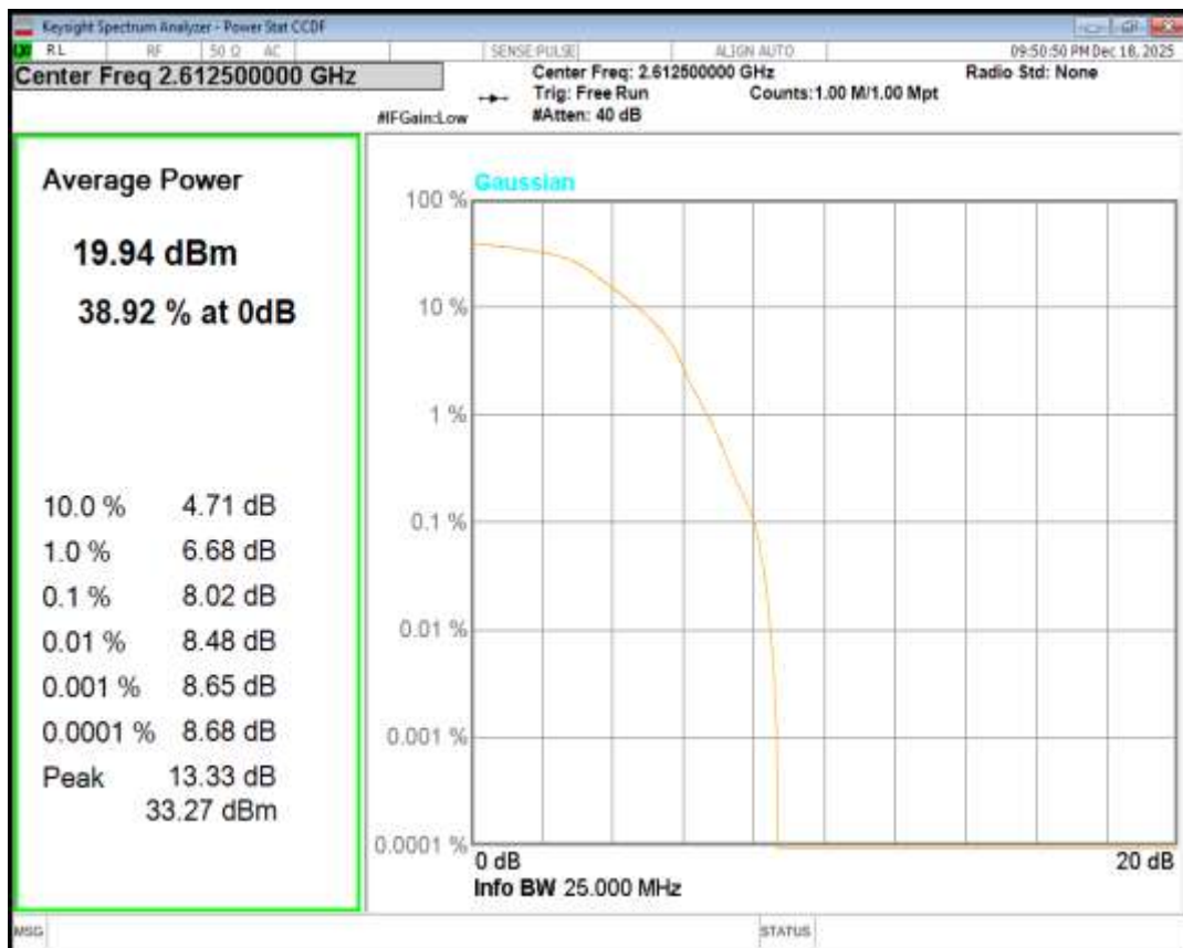
Band38 QPSK BW=20MHz Channel=37850 RB Size=1 Position=#0
