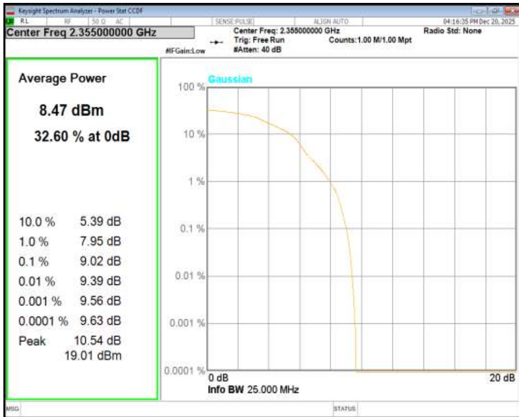
Band40(2350-2360) 16QAM BW=5MHz Channel=39225 RB Size=1 Position=#0
