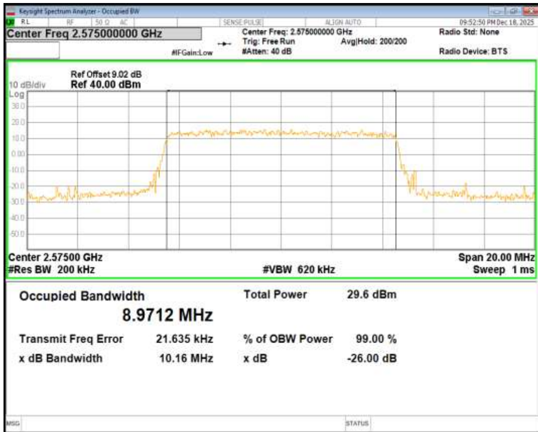
Band38 QPSK BW=10MHz Channel=38000 RB Size=50 Position=#0
