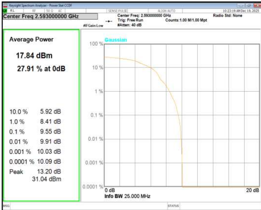
Band41 16QAM BW=5MHz Channel=41565 RB Size=1 Position=#0
