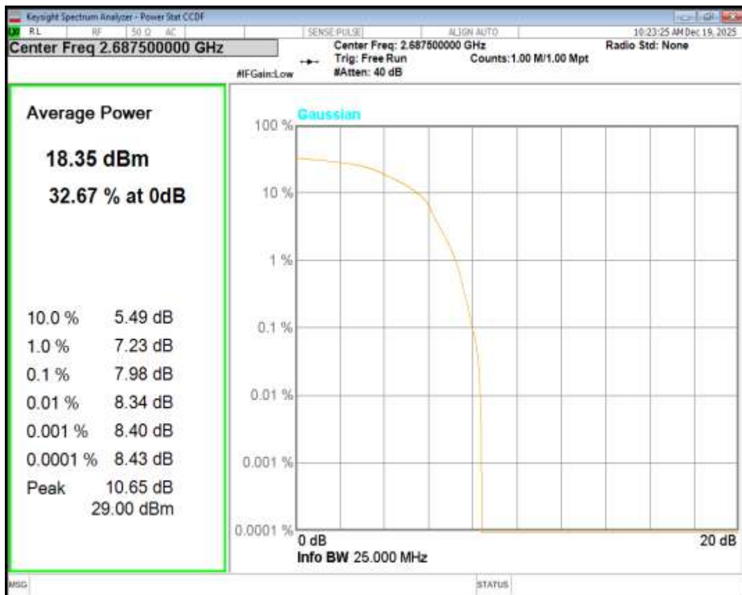
Band41 QPSK BW=10MHz Channel=39700 RB Size=1 Position=#0
