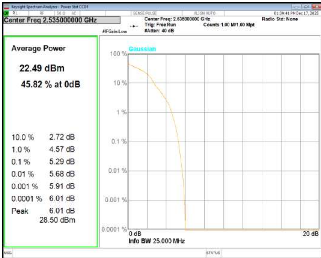
Band7 16QAM BW=5MHz Channel=21425 RB Size=1 Position=#0
