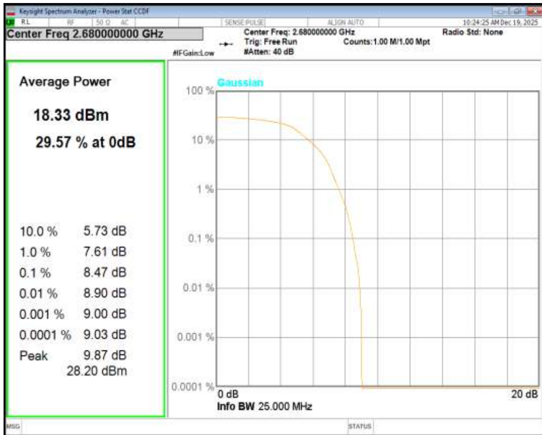
Band41 QPSK BW=5MHz Channel=39675 RB Size=1 Position=#0
