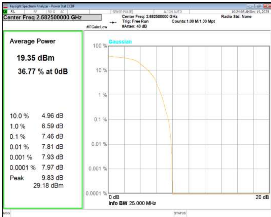
Band41 QPSK BW=20MHz Channel=39750 RB Size=1 Position=#0
