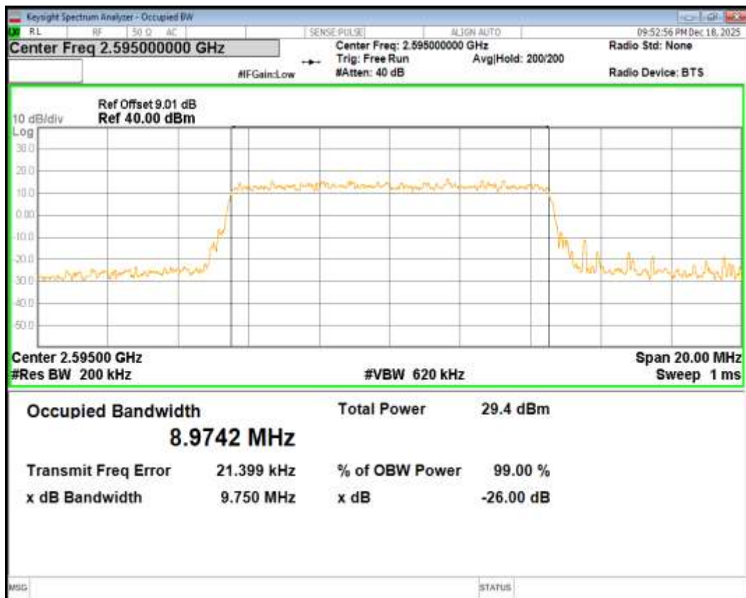
Band38 QPSK BW=10MHz Channel=38200 RB Size=50 Position=#0
