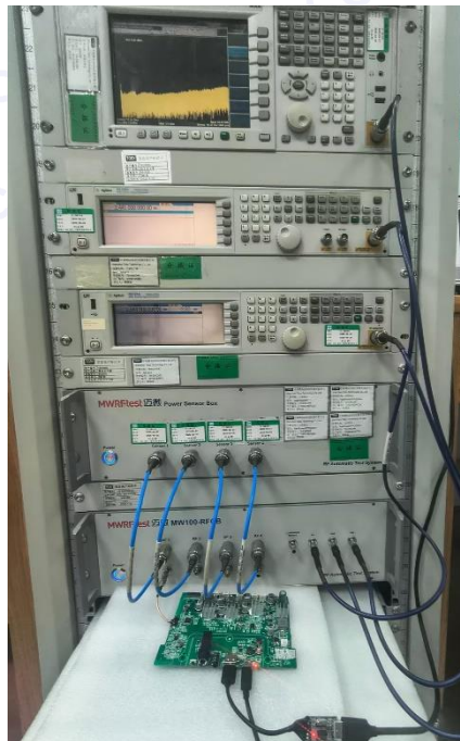
Photo of Setup for Conducted Measurements
