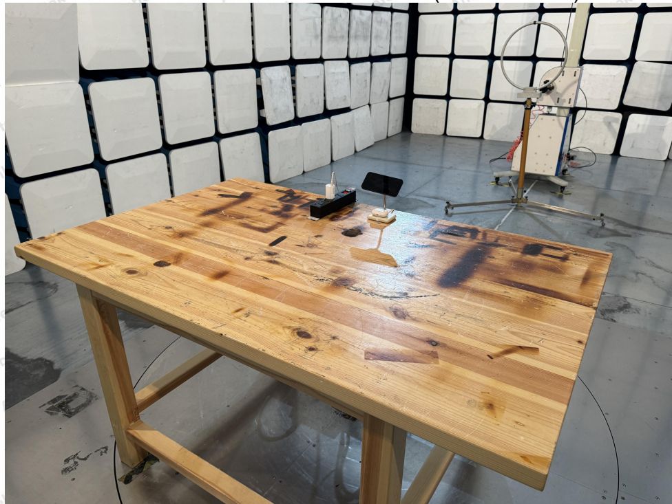
Photo of Radiation Emission Test (below 30MHz)
