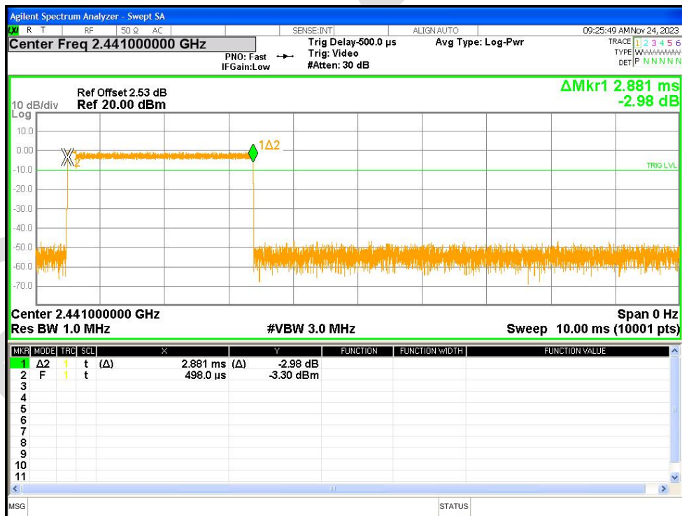
Dwell NVNT 3-DH5 2441MHz Ant1 Accumulated
