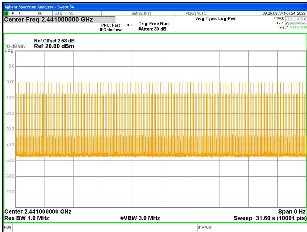
Dwell NVNT 3-DH5 2441MHz Ant1 One Burst
