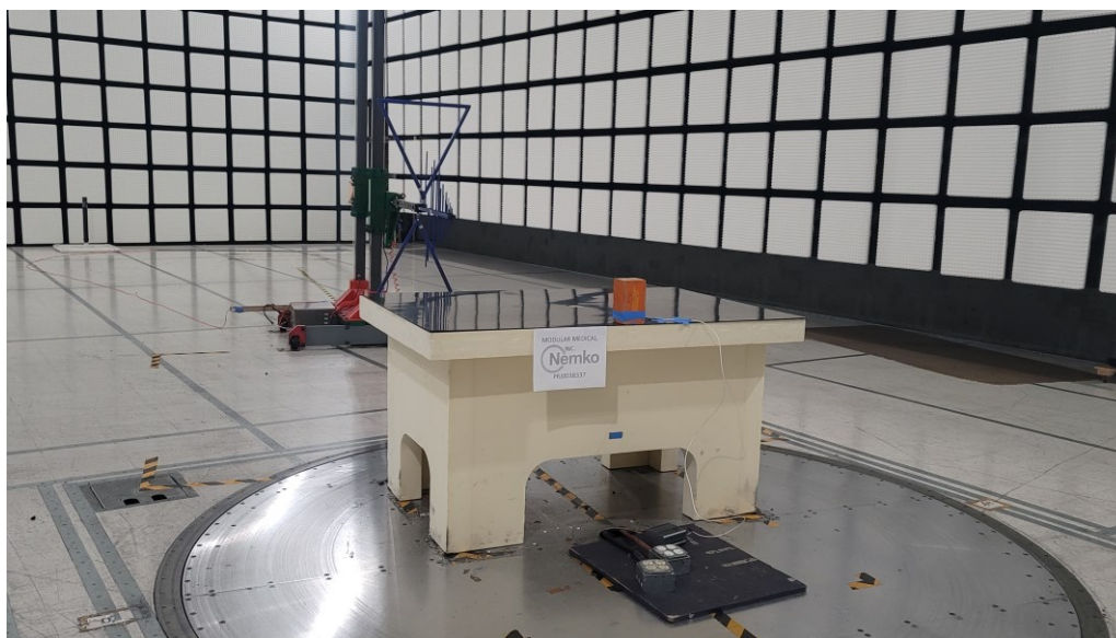
Figure 3 - Radiated emissions below 1 GHz (0.03 – 1 GHz), rear view.
