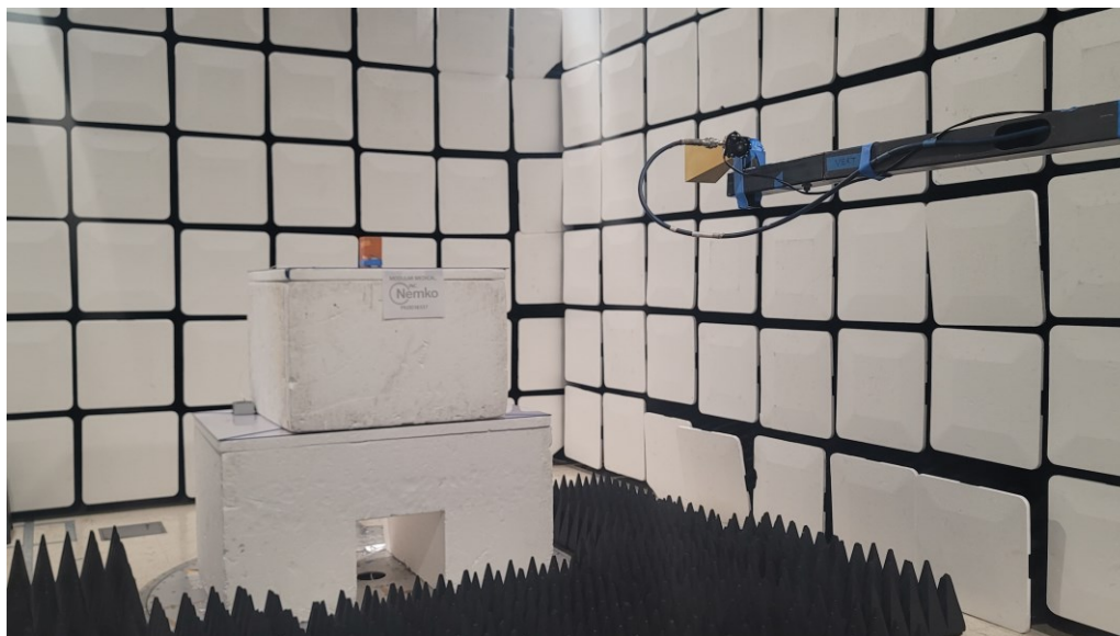
Figure 6 - Radiated emissions above 1 GHz (18 – 26.5 GHz), front view.
