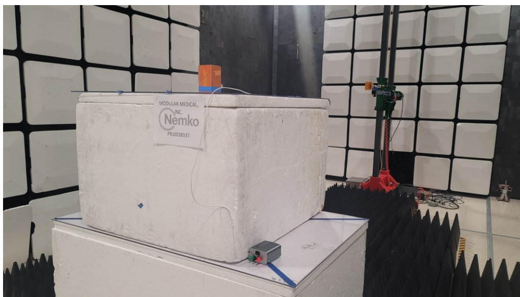
Figure 7 - Radiated emissions above 1 GHz (18 – 26.5 GHz).
