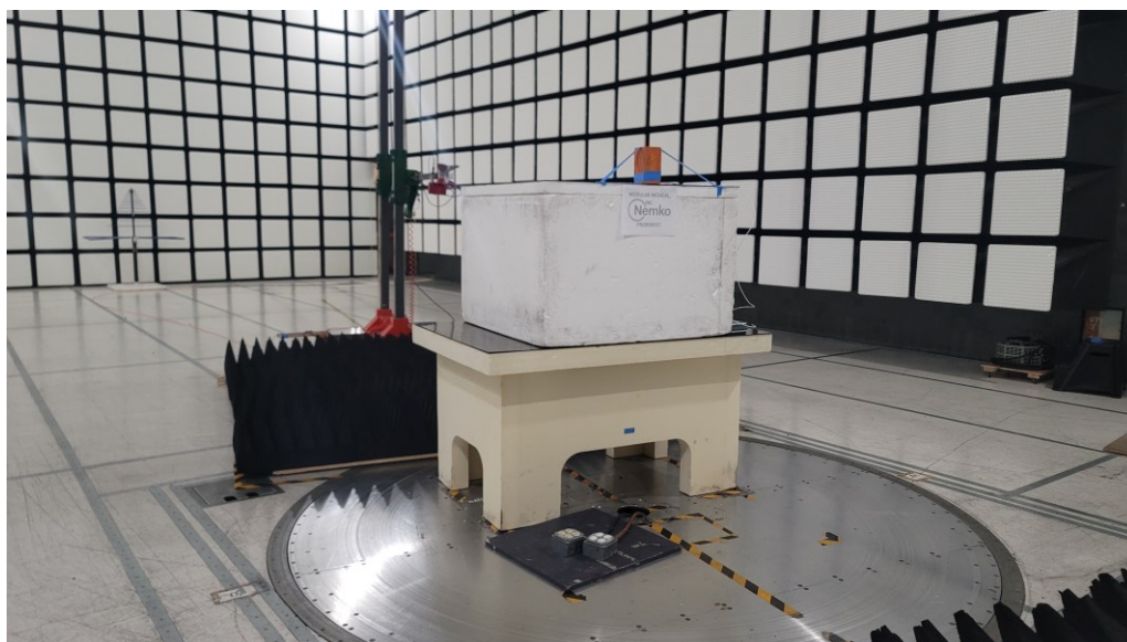
Figure 5 - Radiated emissions above 1 GHz (1 – 18 GHz), rear view.
