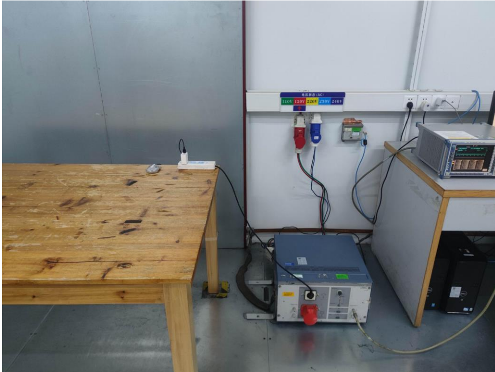
AC POWER LINE CONDUCTED TEST SETUP
