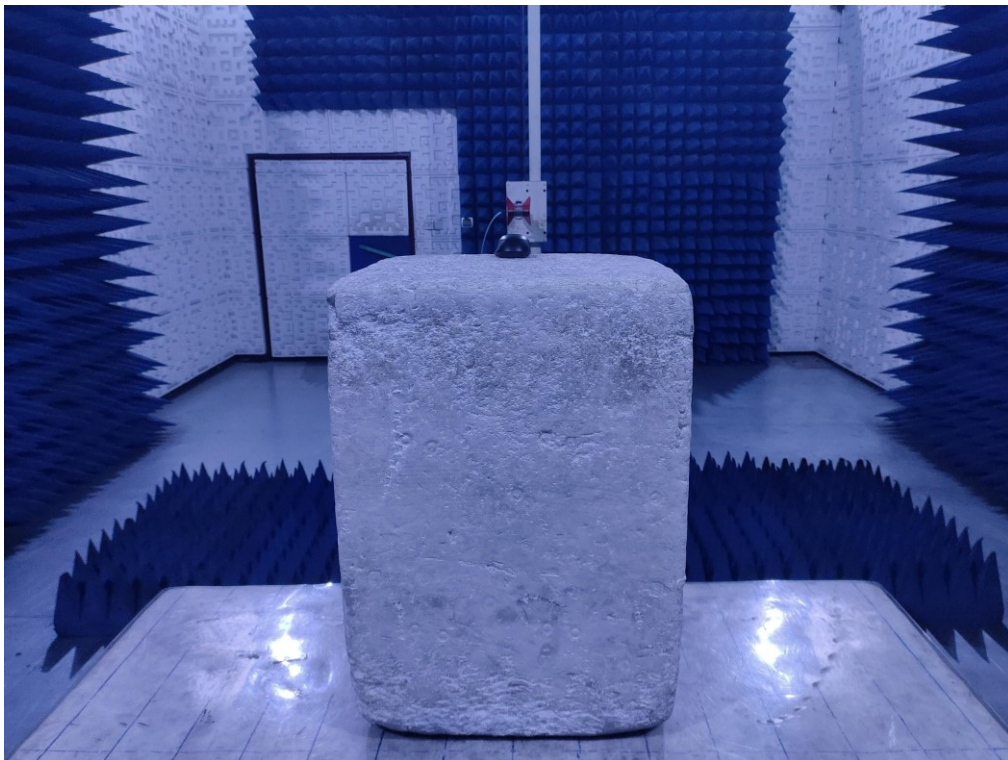
RADIATED EMISSION TEST SETUP ABOVE 1GHz
