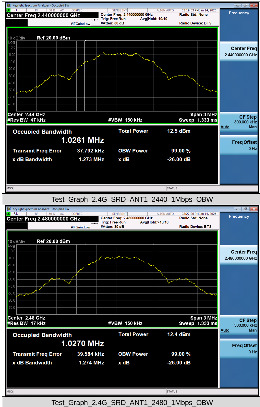
Test Graphs of DTS Bandwidth
