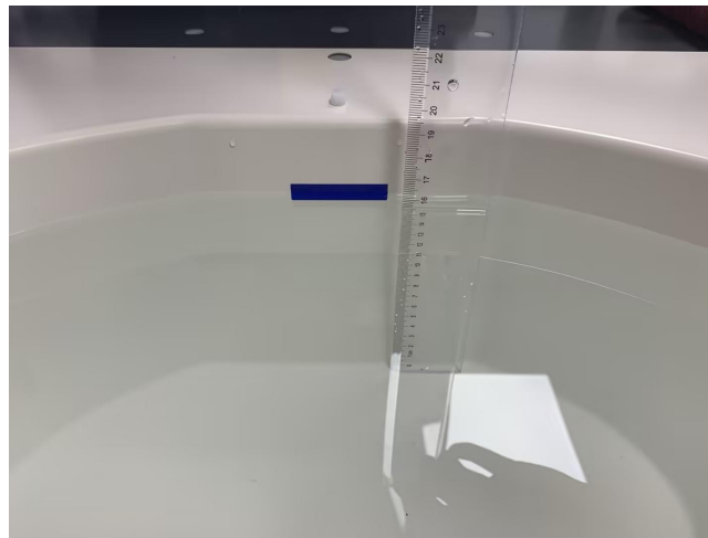
Liquid Height for Body SAR
