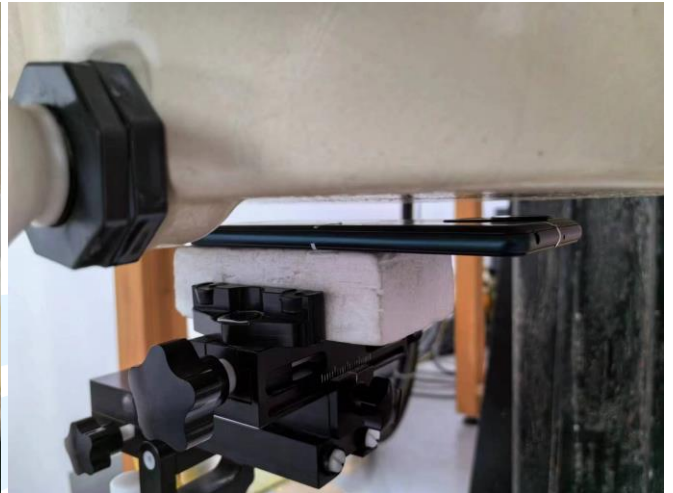
Rear Face of EUT with 1 cm Gap
