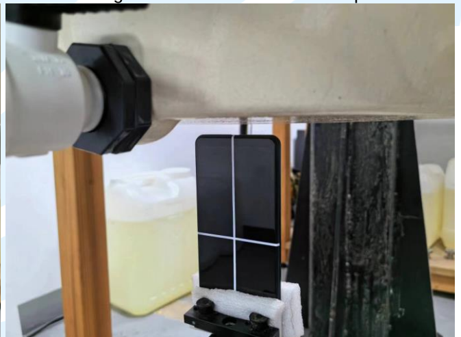
Bottom Side of EUT with 1 cm Gap
