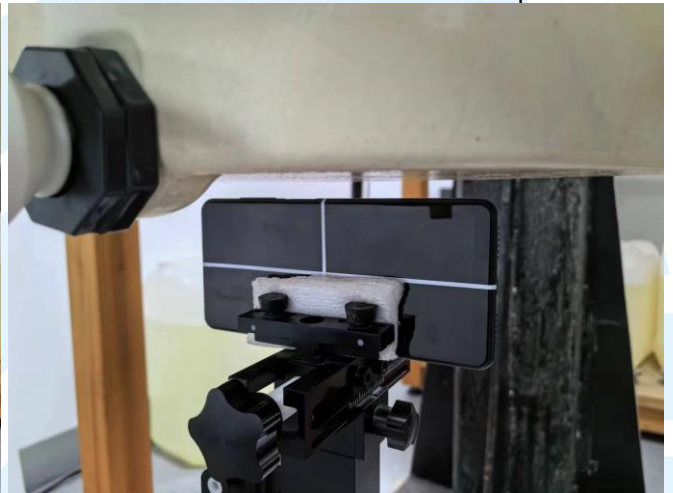
Right Side of EUT with 1 cm Gap
