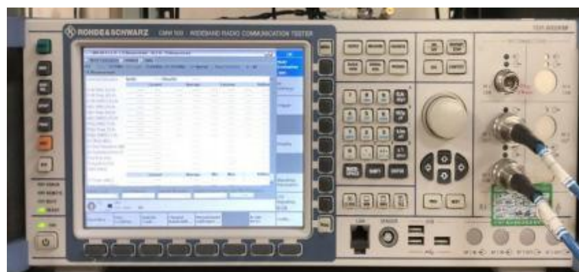
CMW 500 (2G/3G/4G Test Equipment)
