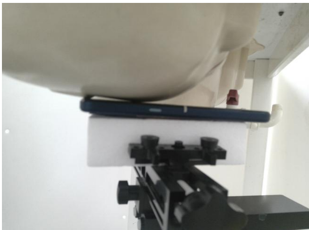
Right Cheek, Test Separation 0 mm
