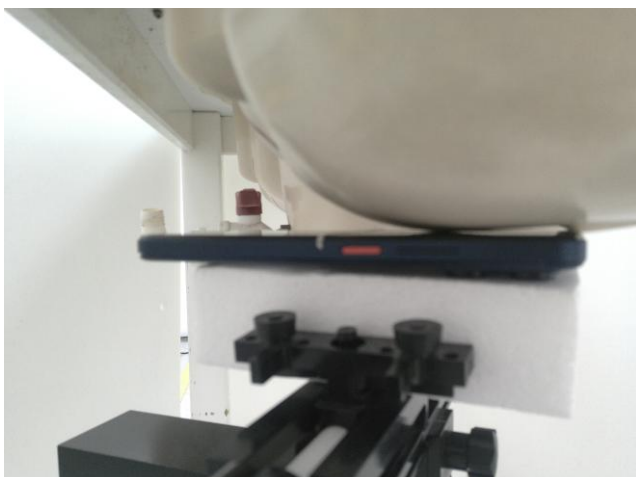
Left Cheek, Test Separation 0 mm
