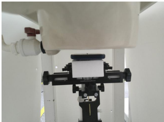
Front, Test Separation 10 mm
