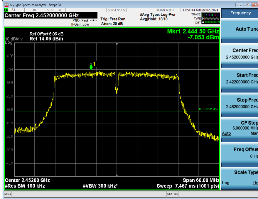
1 Reference Level NVNT_ANT2_802_11n(HT40)_2452
