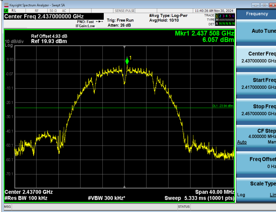
2 Spurious Emission NVNT_ANT1_802_11b_2437
