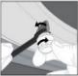
(Fig. c) Use the wrench tool to tighten the anti-theft nut counterclockwise to secure the sensor
