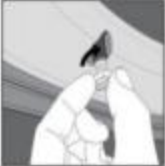
(Fig. a) Clockwise screw the anti-theft nut to the bottom of the tire valve.
