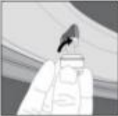
(Fig. b) Quickly tighten the sensor clockwise. Air leakage during installation is normal and will stop once the sensor is fully tightened.
