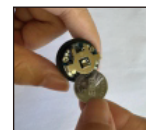
c. Put in a new battery, screw the top cover and instal it to the air nozzle (the battery has words facing up)
