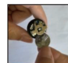
c Insert the new battery and screw the cover on, then install it onto the valve stem (battery text side facing up)
