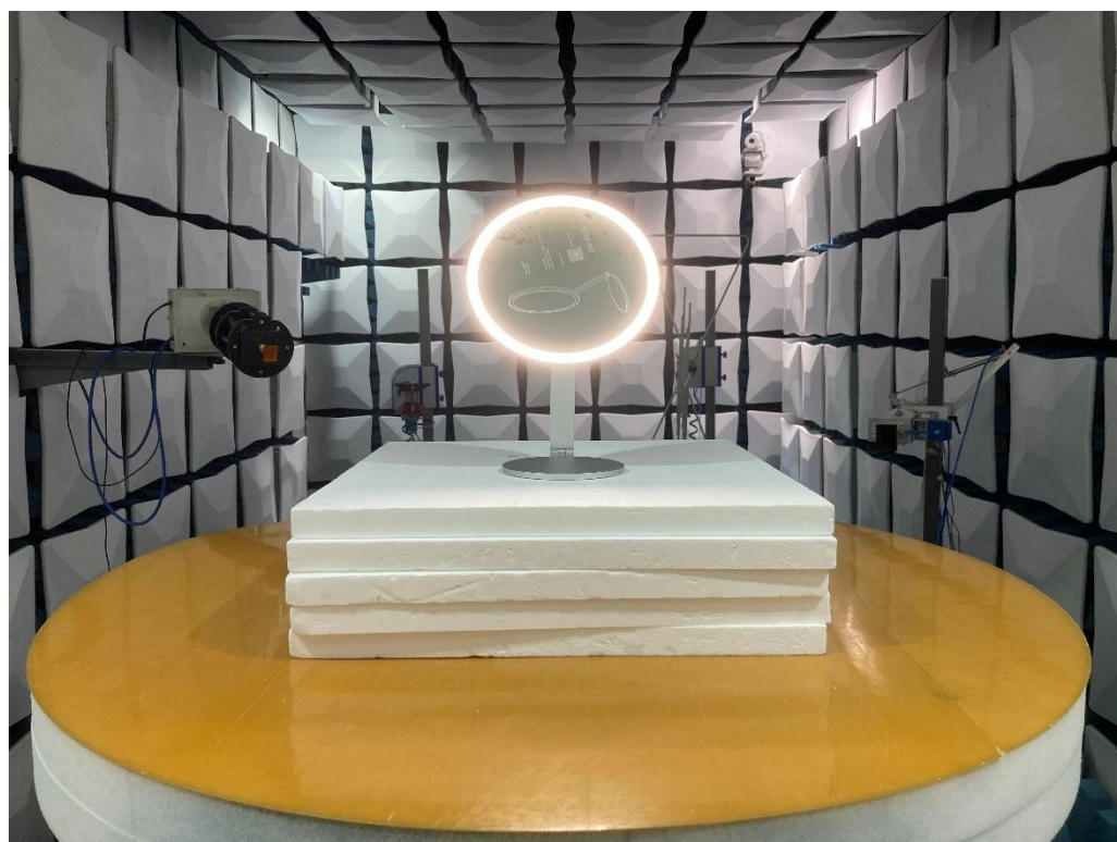
Photograph 4: Set-up photo for Radiated Spurious Emission, above 40GHz
