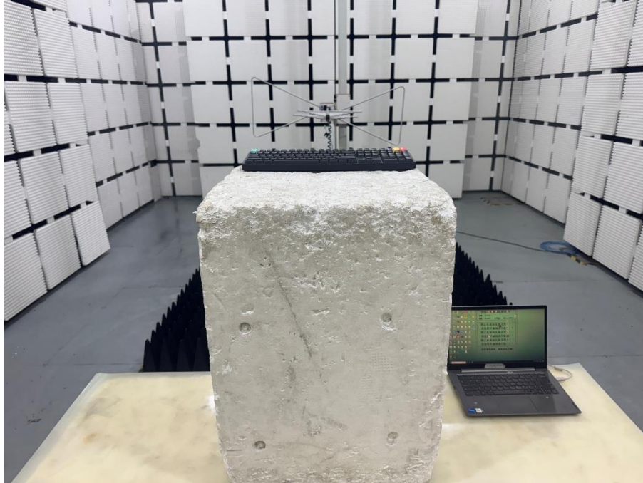
Set-up for Radiated Spurious Emission, Above 1GHz
