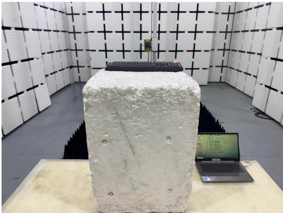
Set-up for Radiated Spurious Emission, Above 1GHz
