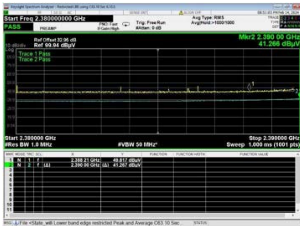
Figure 50 – Band-edge Measurement, WiFi G, High Data Rate, Low Channel, Restricted Frequency
