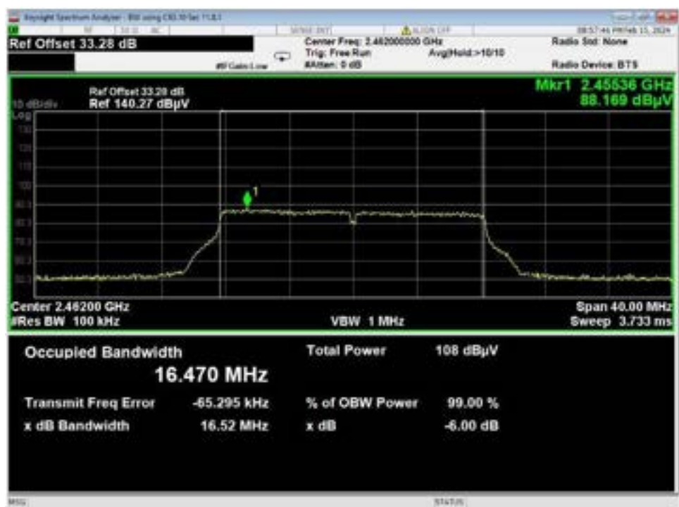
Figure 34 - Bandwidth, WiFi G, Low Data Rate, High Channel
