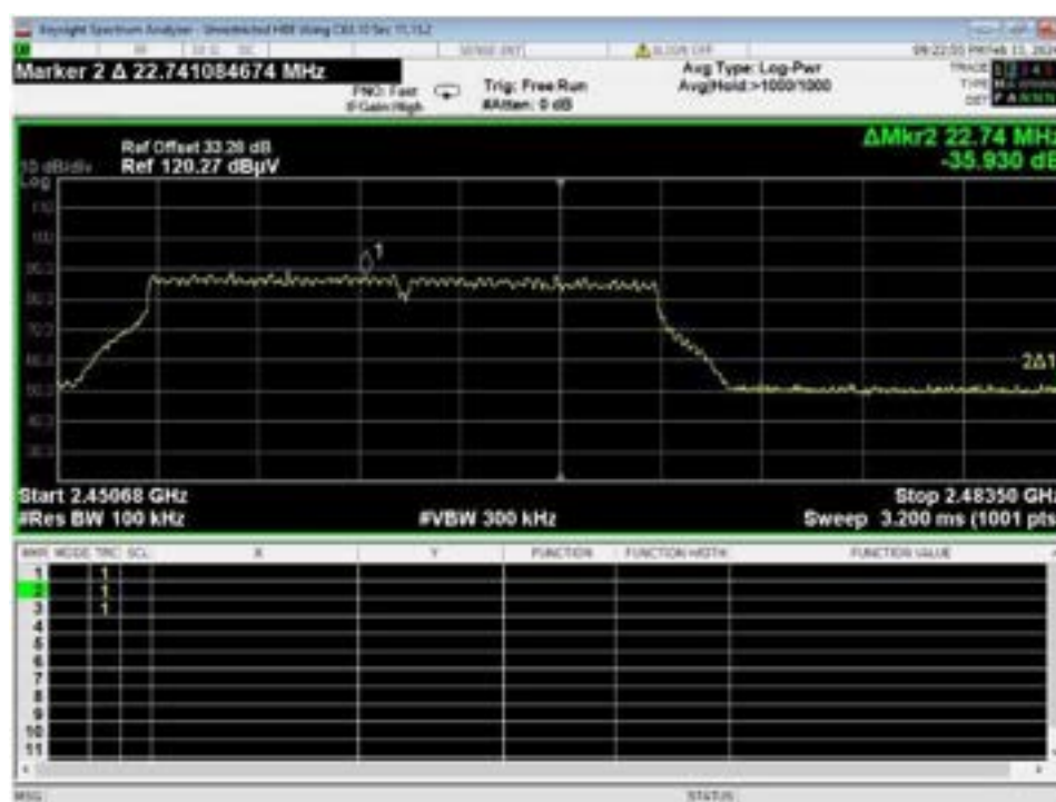
Figure 63 – Band-edge Measurement, WiFi G, High Data Rate, High Channel, Unrestricted Frequency
