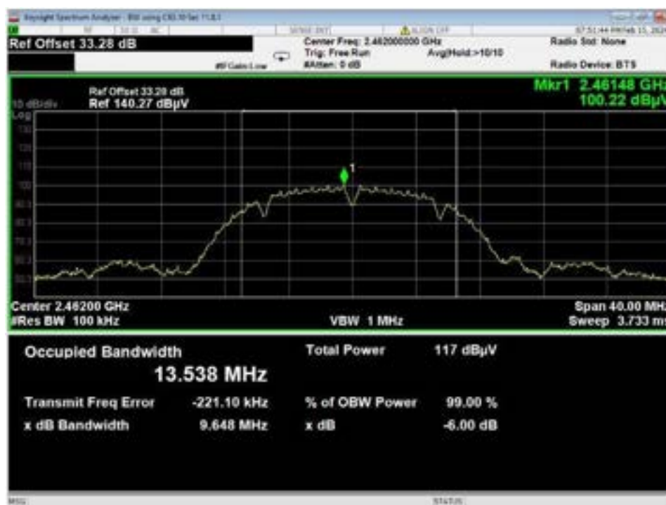
Figure 28 - Bandwidth, WiFi B, Low Data Rate, High Channel
