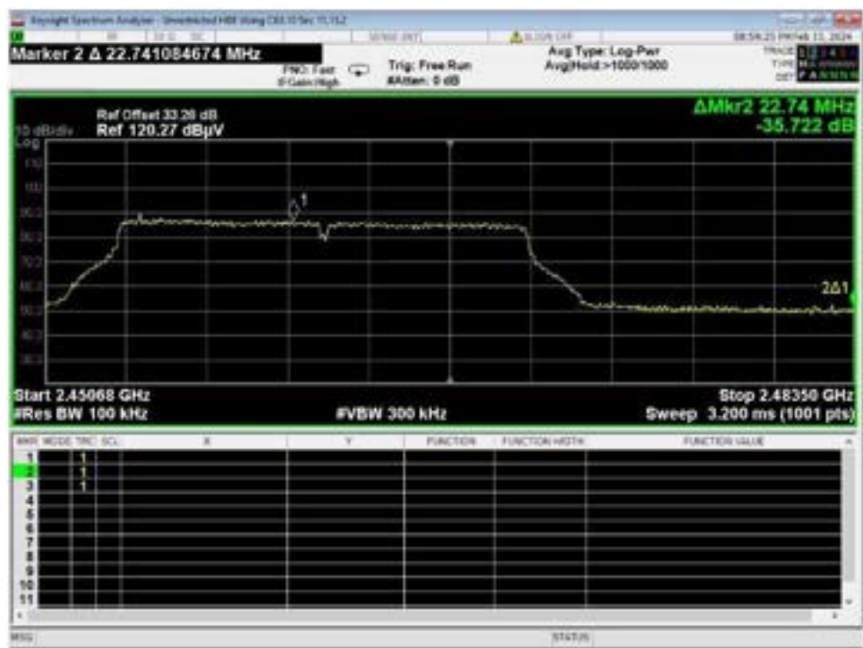
Figure 61 – Band-edge Measurement, WiFi G, Low Data Rate, High Channel, Unrestricted Frequency
