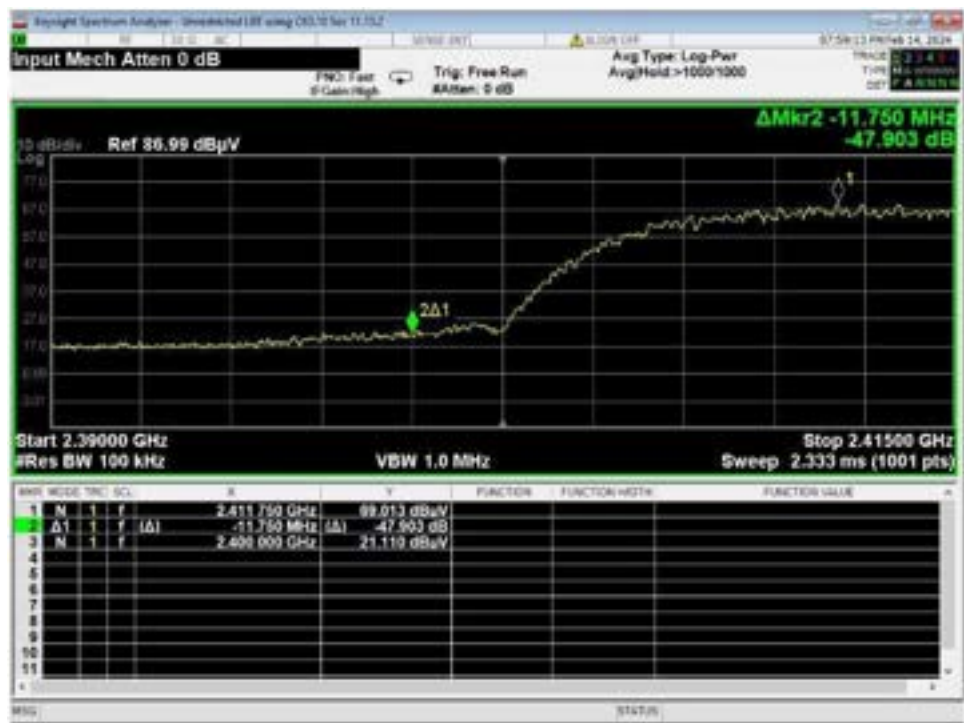
Figure 58 – Band-edge Measurement, WiFi B, High Data Rate, Low Channel, Unrestricted Frequency
