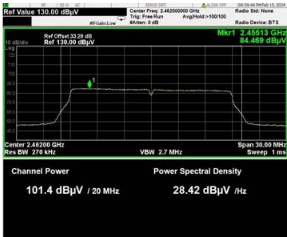
Figure 21 – Radiated Output Power Field Strength, WiFi N, Low Data Rate, High Channel
