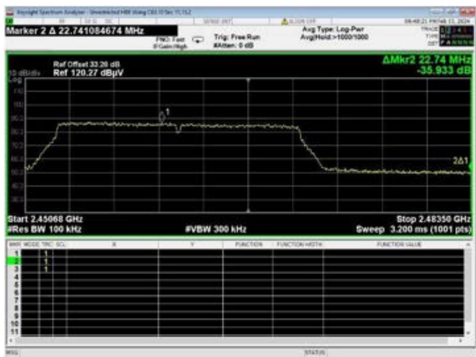
Figure 65 – Band-edge Measurement, WiFi N, Low Data Rate, High Channel, Unrestricted Frequency
