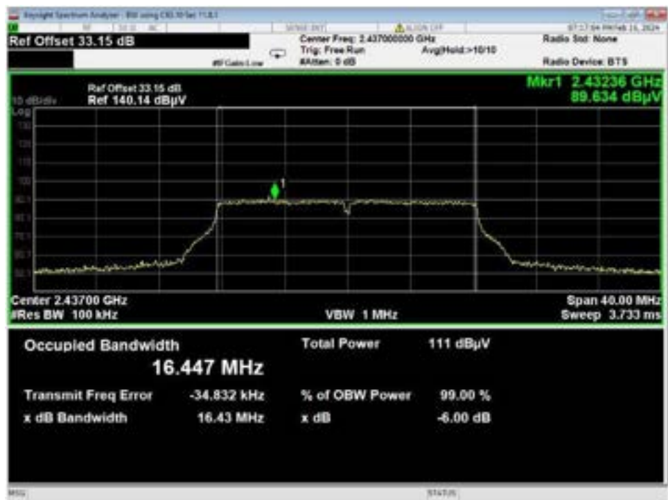
Figure 33 - Bandwidth, WiFi G, Low Data Rate, Mid Channel
