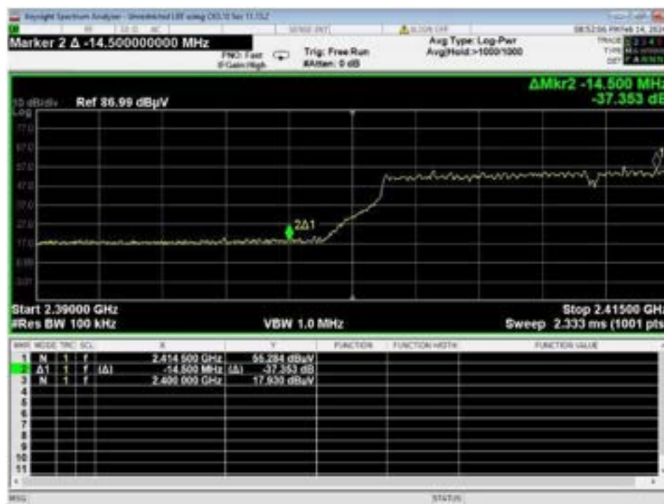
Figure 62 – Band-edge Measurement, WiFi G, High Data Rate, Low Channel, Unrestricted Frequency
