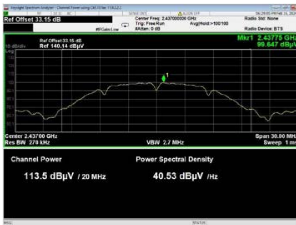
Figure 8 – Radiated Output Power Field Strength, WiFi B, Low Data Rate, Mid Channel
