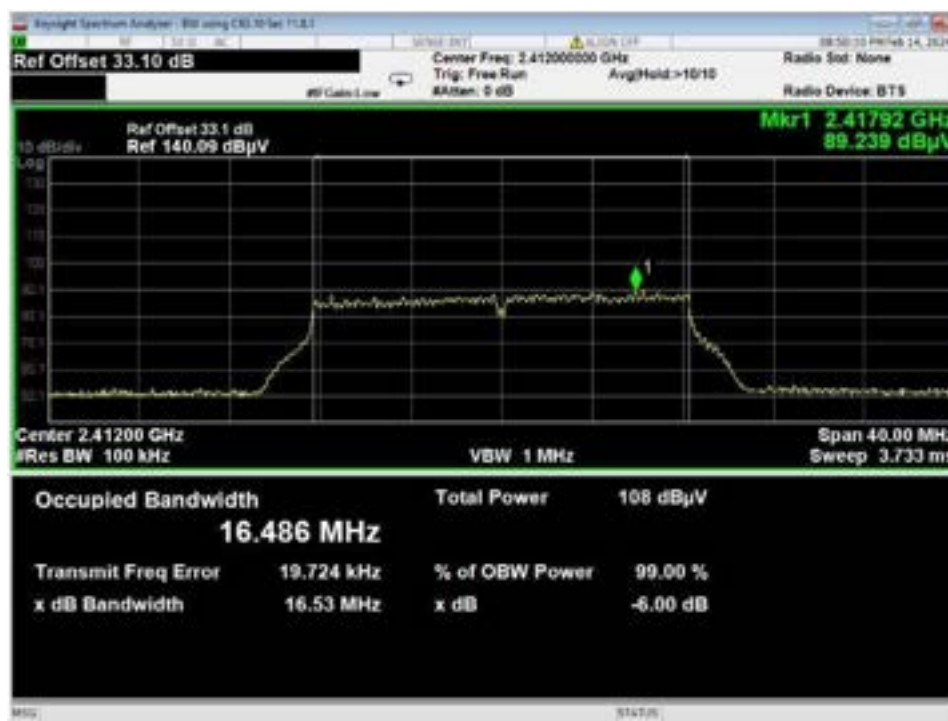
Figure 35 –Bandwidth, WiFi G, High Data Rate, Low Channel
