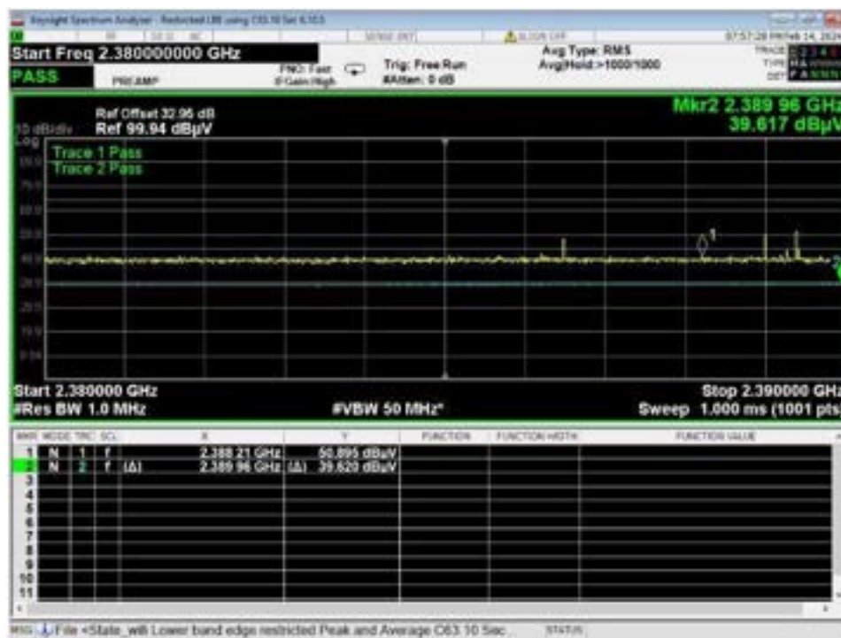
Figure 46 – Band-edge Measurement, WiFi B, High Data Rate, Low Channel, Restricted Frequency
