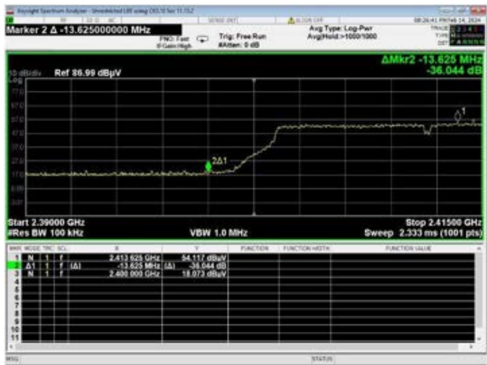
Figure 60 – Band-edge Measurement, WiFi G, Low Data Rate, Low Channel, Unrestricted Frequency
