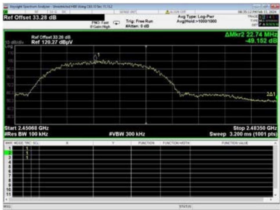
Figure 59 – Band-edge Measurement, WiFi B, High Data Rate, High Channel, Unrestricted Frequency
