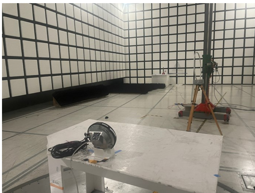
Figure 4 - Radiated emissions below 1 GHz (9k-30MHz), rear view.90 degree
