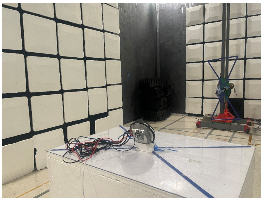
Figure 6 - Radiated emissions below 1 GHz (0.03 – 1 GHz), rear view.
