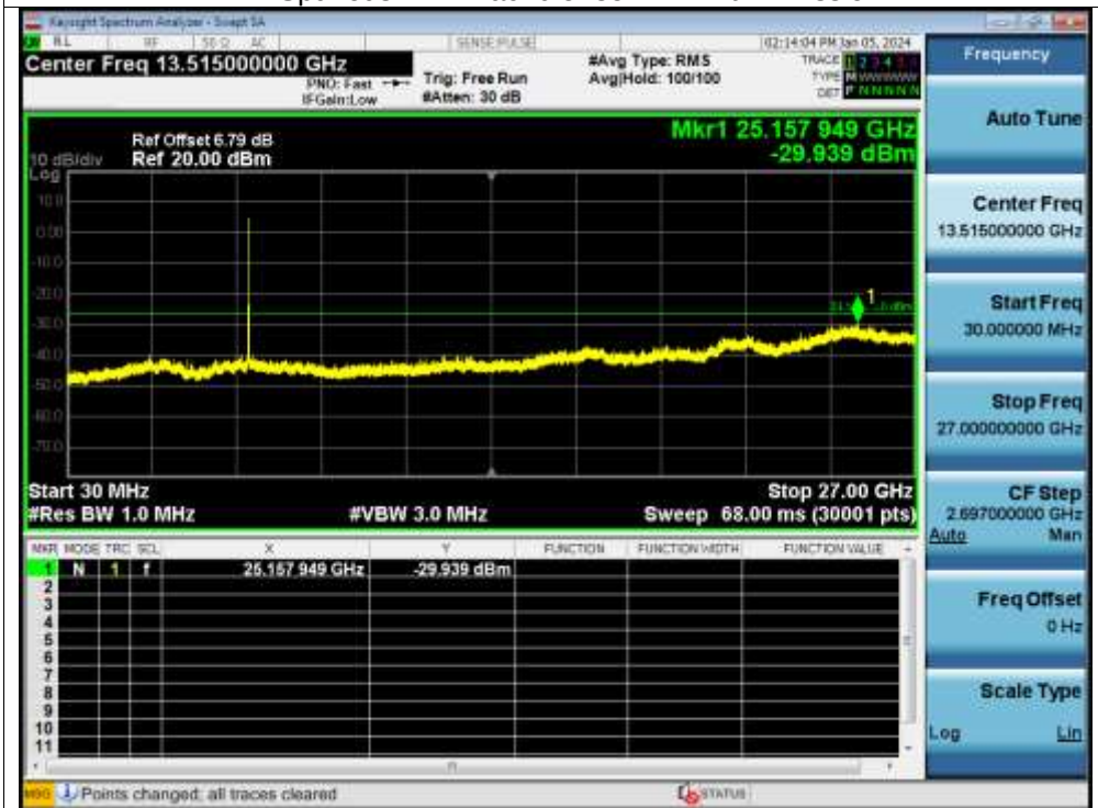
Tx. Spurious NVNT ac20 5785MHz Ant1 Emission
