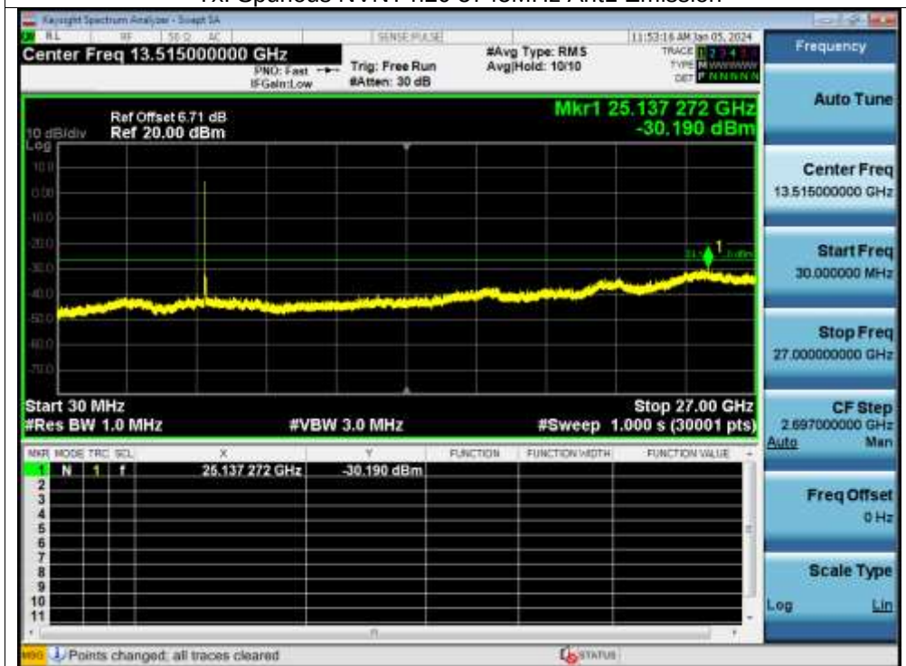
Tx. Spurious NVNT n20 5745MHz Ant1 Emission
