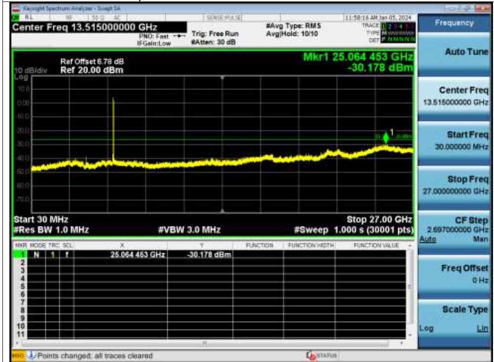
Tx. Spurious NVNT n20 5825MHz Ant1 Emission
