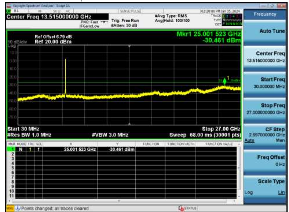
Tx. Spurious NVNT n40 5795MHz Ant1 Emission
