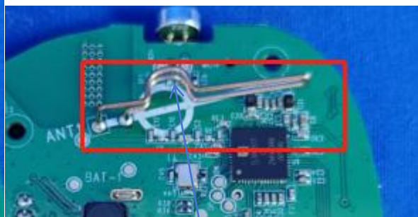
Copper wire Antenna
