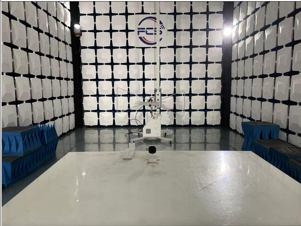
Above 1GHz for radiated emission test setup
