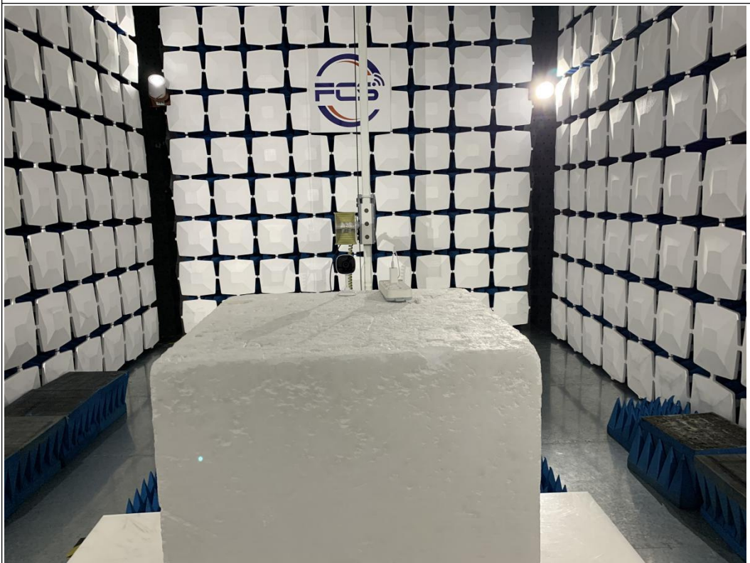
Above 1GHz for radiated emission test setup
