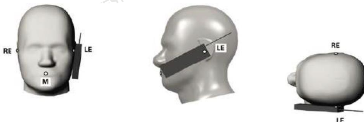
Fig.8-3 Illustration for Cheek Position
