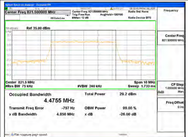
B26 Part90 / 5MHz / 16QAM/ High CH
