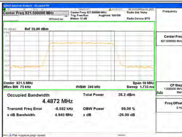
B26 Part90 / 5MHz / 64QAM/ High CH
