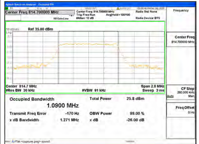
B26 Part90 / 1.4MHz / 256QAM/ Low CH
