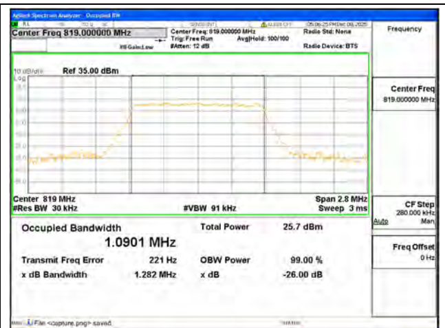
B26 Part90 / 1.4MHz / 256QAM/ Mid CH
