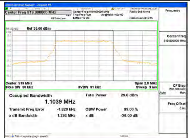
B26 Part90 / 1.4MHz / 16QAM/ Mid CH
