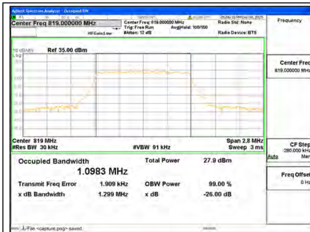
B26 Part90 / 1.4MHz / 64QAM/ Mid CH
