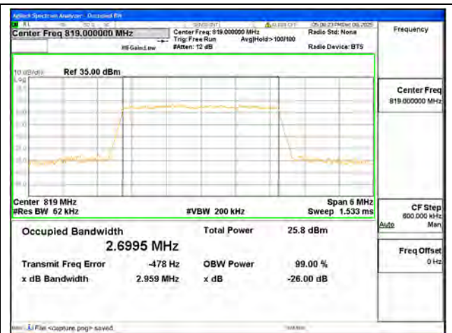
B26 Part90 / 3MHz / 256QAM/ Mid CH
