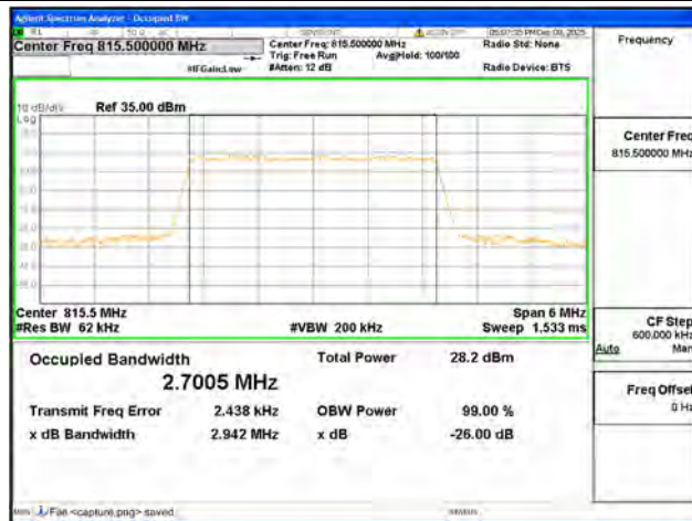
B26 Part90 / 3MHz / 64QAM/ Low CH
