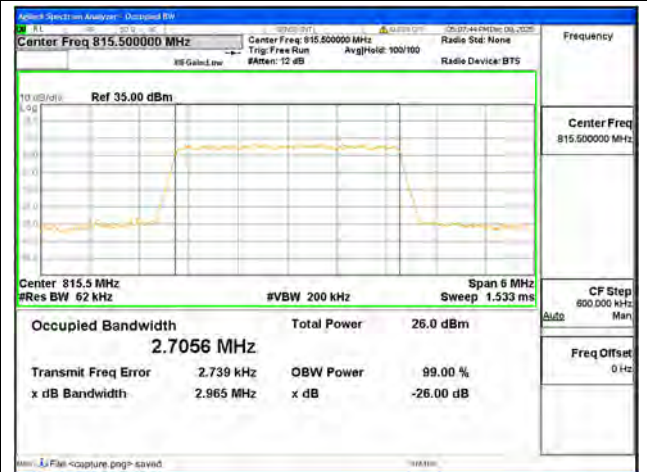
B26 Part90 / 3MHz / 256QAM/ Low CH
