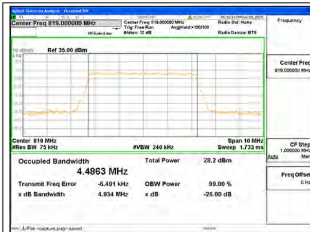
B26 Part90 / 5MHz / 64QAM/ Mid CH
