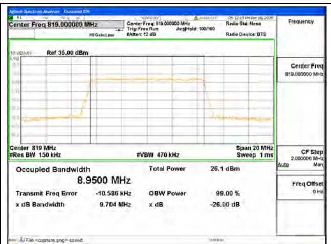
B26 Part90 / 10MHz / 256QAM/ Mid CH
