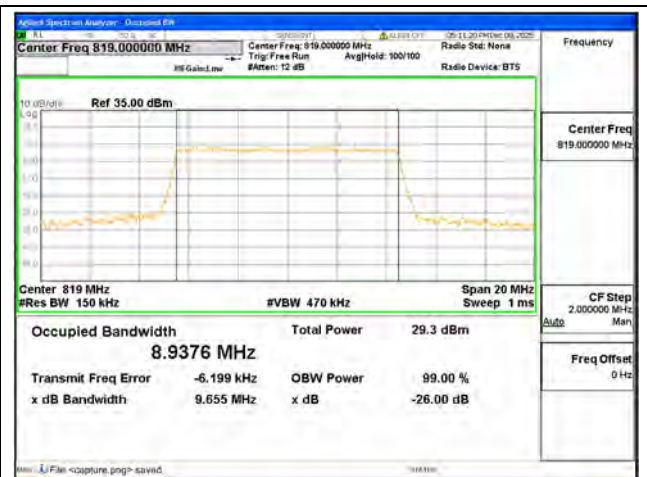
B26 Part90 / 10MHz / 16QAM/ Low CH
