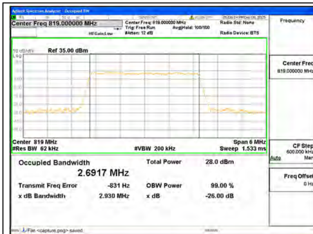
B26 Part90 / 3MHz / 64QAM/ Mid CH
