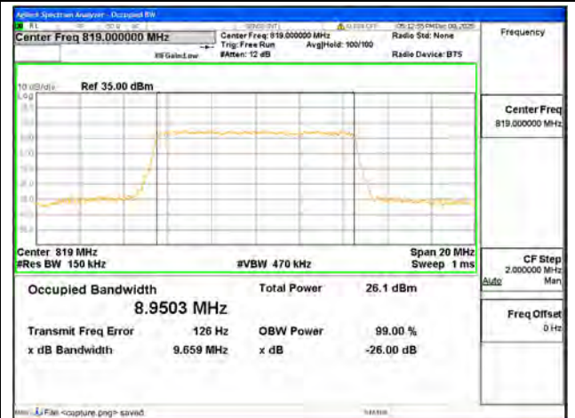
B26 Part90 / 10MHz / 256QAM/ High CH
