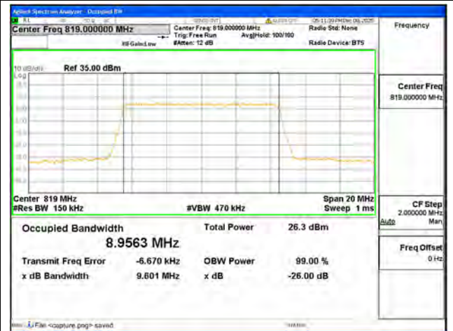
B26 Part90 / 10MHz / 256QAM/ Low CH
