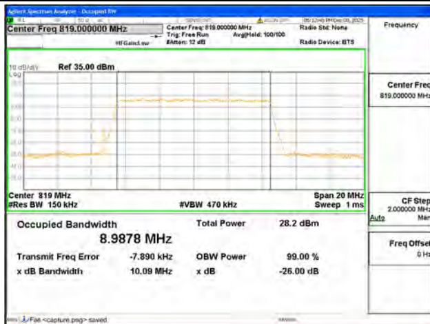
B26 Part90 / 10MHz / 64QAM/ High CH
