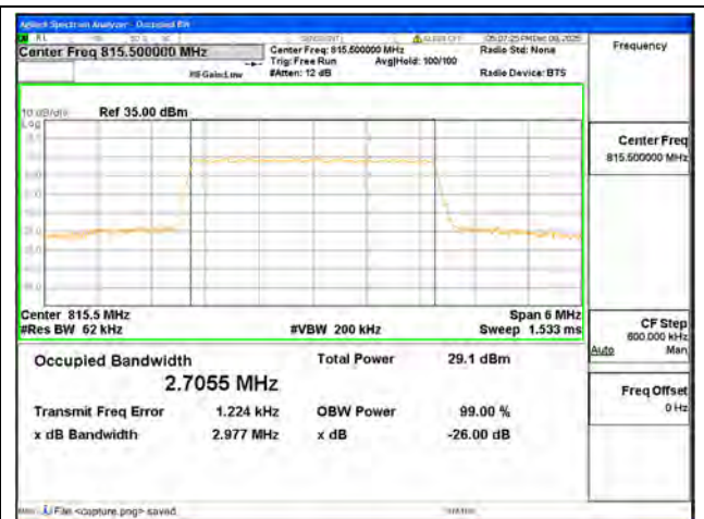
B26 Part90 / 3MHz / 16QAM/ Low CH
