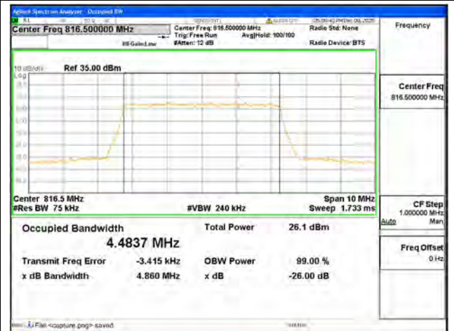
B26 Part90 / 5MHz / 256QAM/ Low CH
