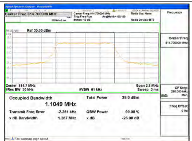
B26 Part90 / 1.4MHz / 16QAM/ Low CH
