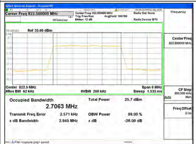
B26 Part90 / 3MHz / 256QAM/ High CH
