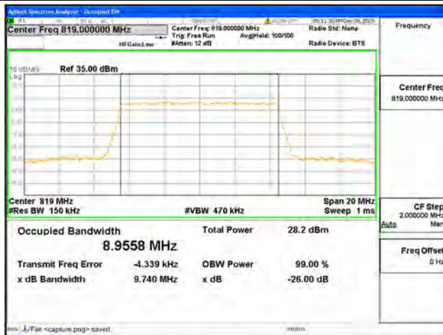
B26 Part90 / 10MHz / 64QAM/ Low CH
