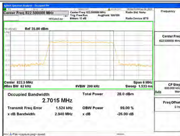
B26 Part90 / 3MHz / 64QAM/ High CH
