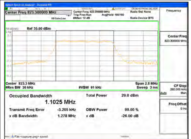
B26 Part90 / 1.4MHz / 16QAM/ High CH
