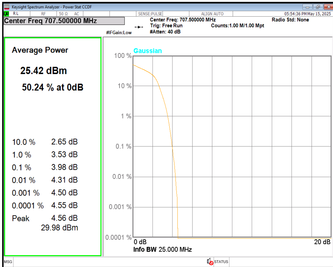
Band12 QPSK BW=10MHz Channel=23130 RB Size=1 Position=#0
