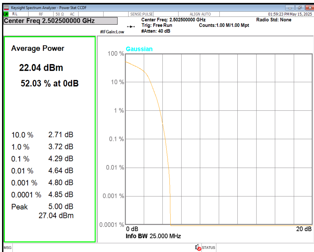
Band7 QPSK BW=5MHz Channel=21100 RB Size=1 Position=#0
