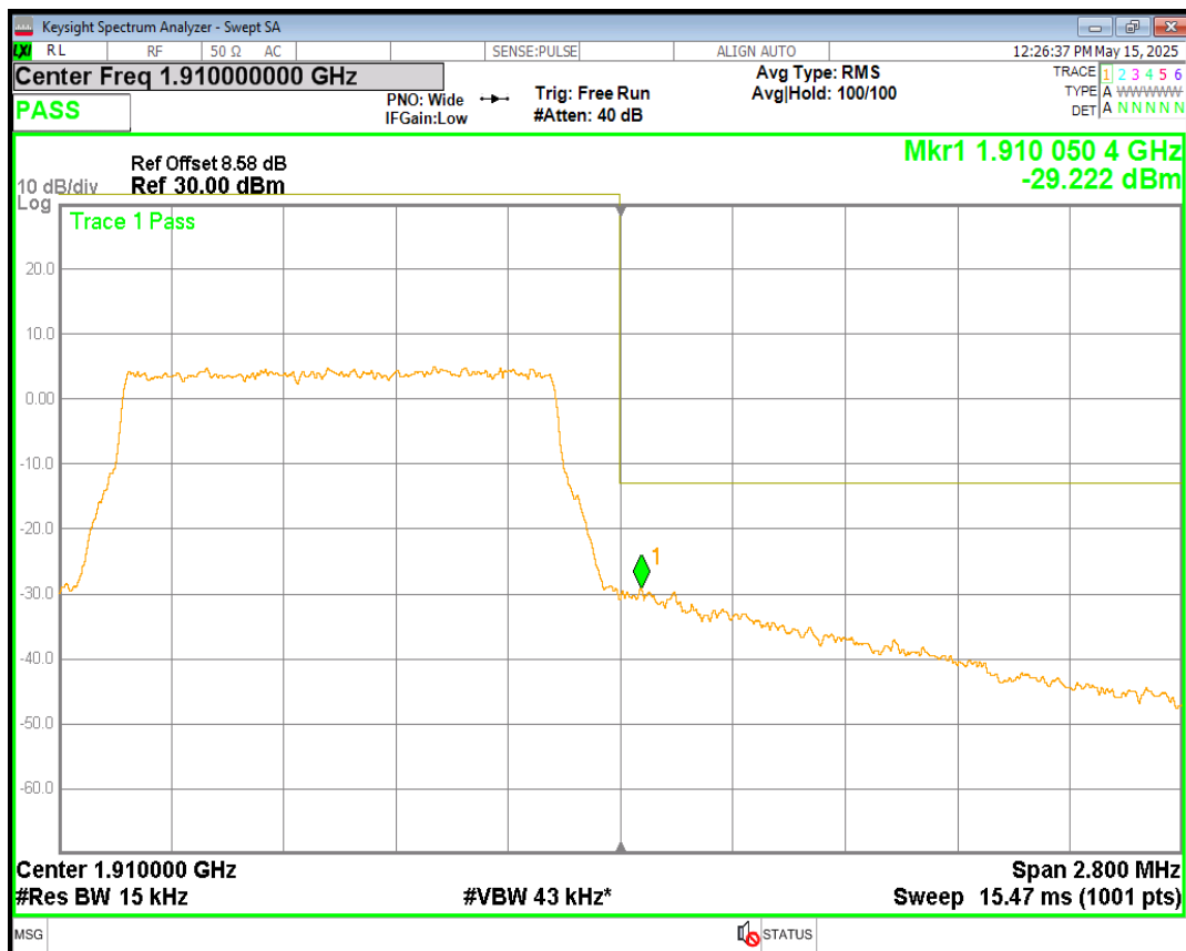
Band2 QPSK BW=3MHz Channel=18615 RB Size=15 Position=#0
