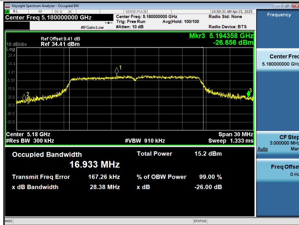
-26dB Bandwidth NVNT a 5180MHz Ant2
