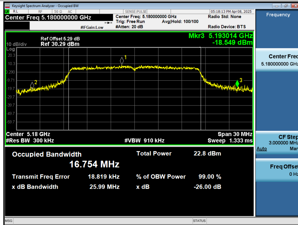
-26dB Bandwidth NVNT a 5180MHz Ant2
