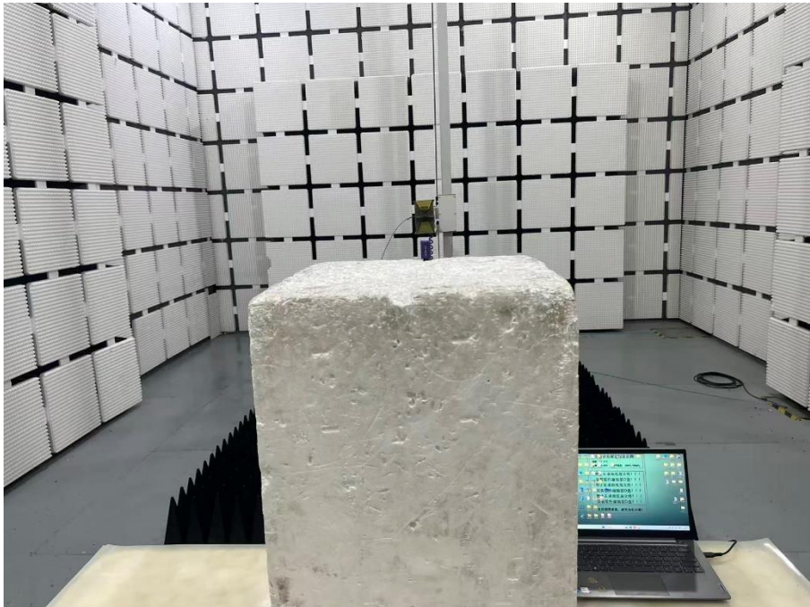
Set-up for Radiated Spurious Emission, Above 1GHz
