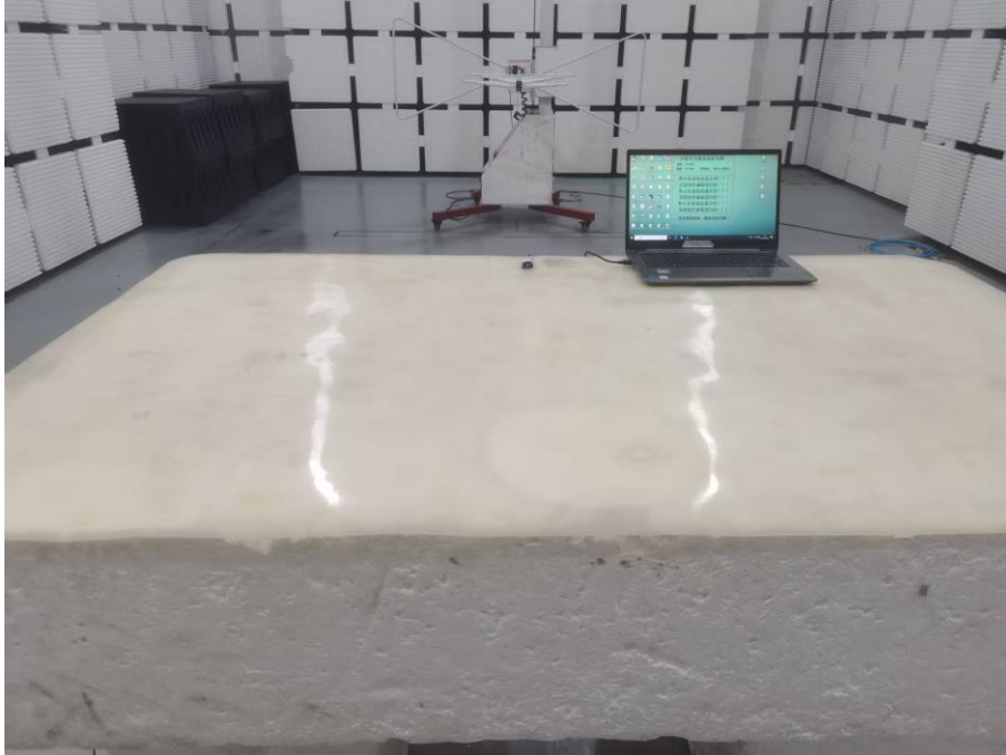
Set-up for Radiated Spurious Emission, Above 1GHz
