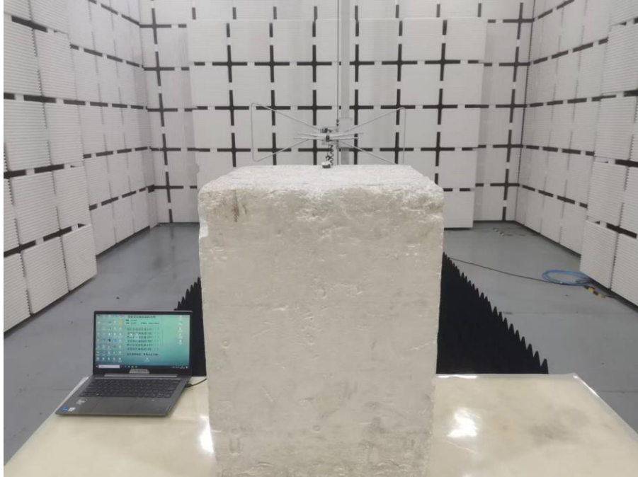
Set-up for Radiated Spurious Emission, Above 1GHz
