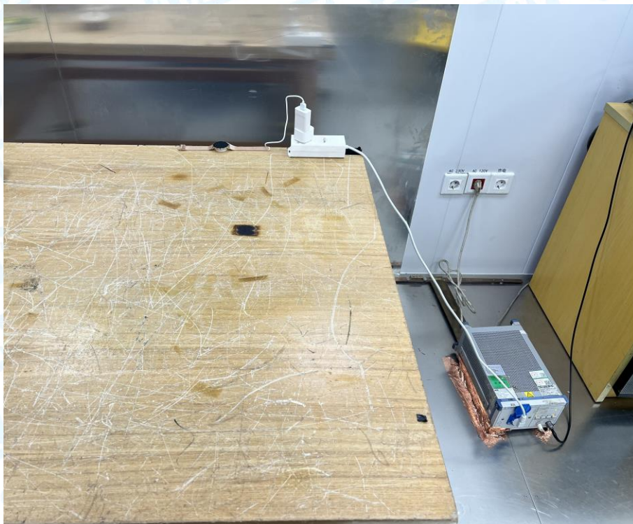
Photo of Setup for Conducted Emission
