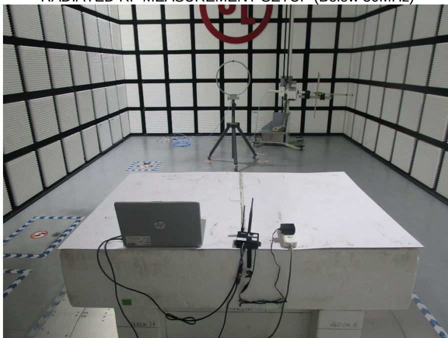
RADIATED RF MEASUREMENT SETUP (Below 30MHz)
